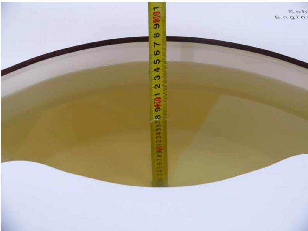
Picture 3 Liquid depth in the Flat Phantom (835 MHz)
