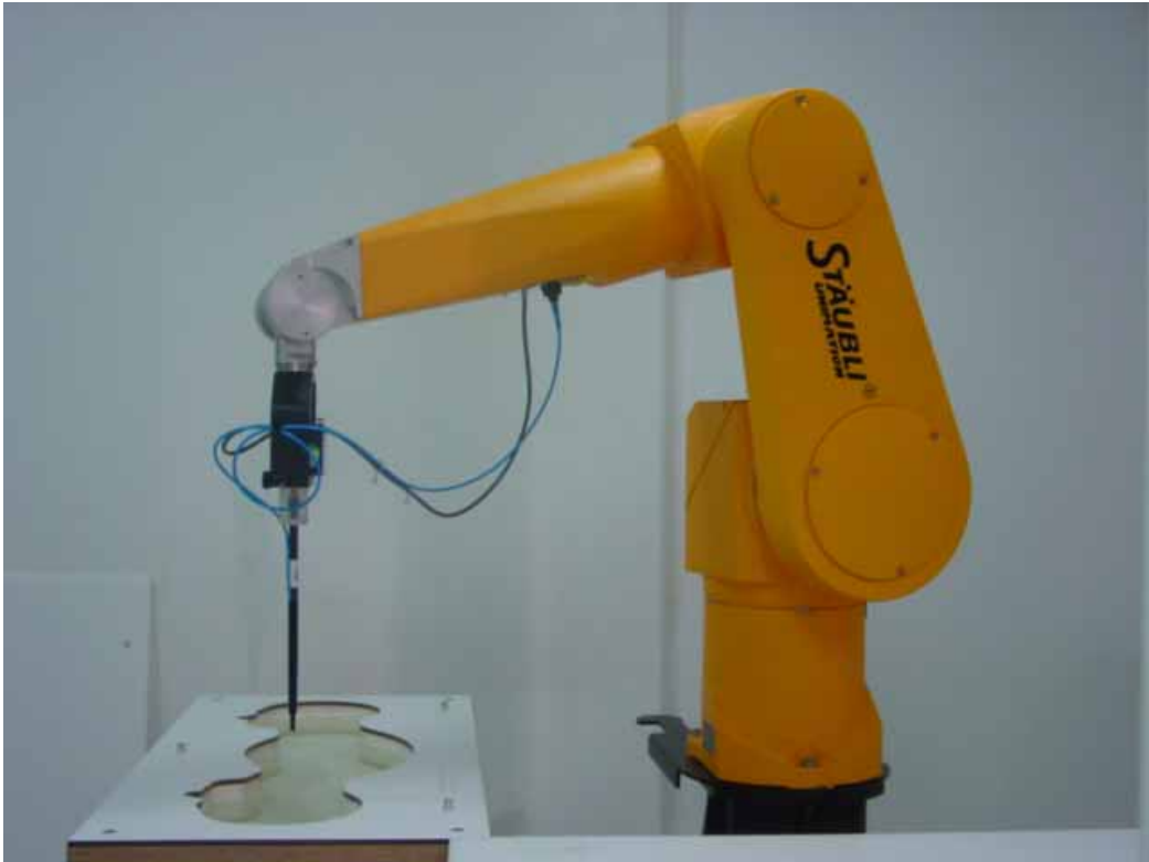
Picture 2 Specific Absorption Rate Test Layout
