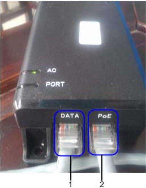
Figure 3-42 Connecting the PoE adapter
