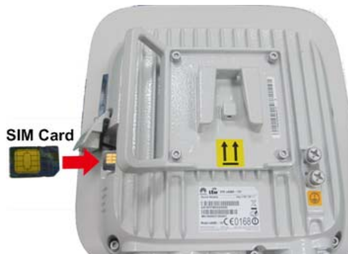
Figure 3-3 Installing the SIM card
