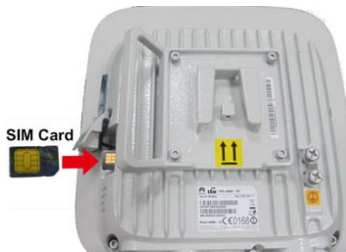
Figure 3-23 Installing the SIM card
