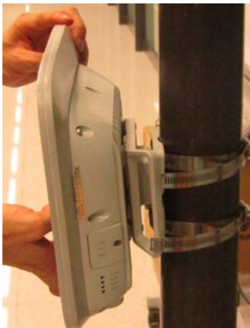
Figure 3-7 Installing the eA660 on the wall-mounting frame
