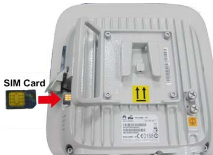
Figure 3-11 Installing the SIM card
