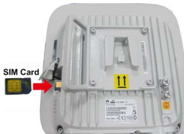
Figure 3-32 Installing the SIM card
