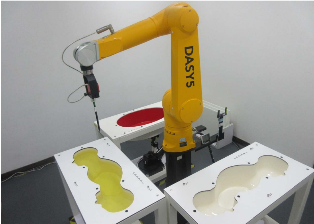
Liquid depth in the flat Phantom ( \geq 15\text{cm} depth)
