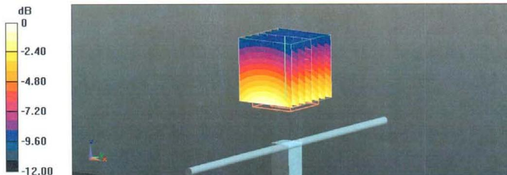
Impedance Measurement Plot for Head TSL
