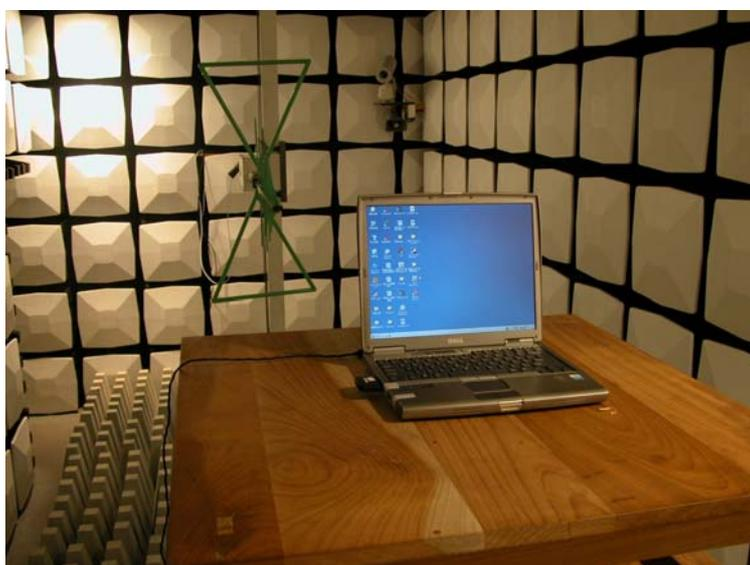
Radiated Spurious Emission (below 1 GHz, without external antenna)
