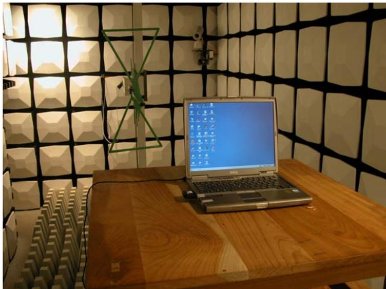
Radiated Spurious Emission (bellow 1 GHz , without external antenna)
