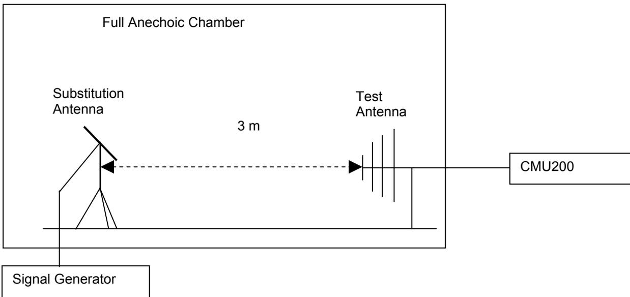
Figure 1. Test Set-up
