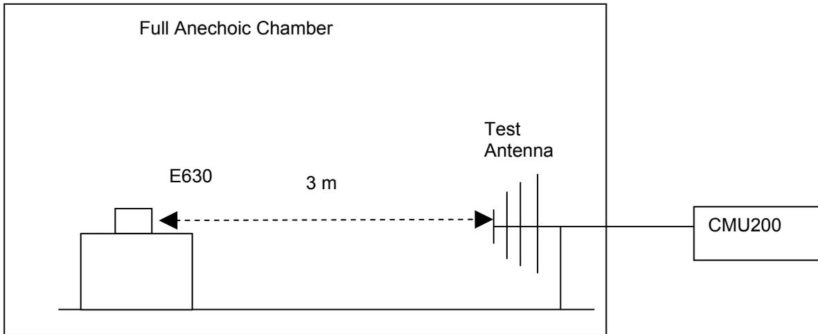
**Step 2: Substitution method to verify the maximum EIRP**
