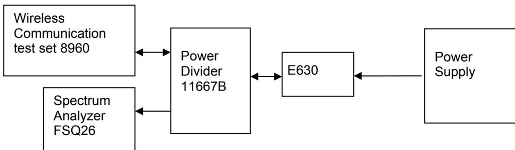
Figure 3. Test Set-up
