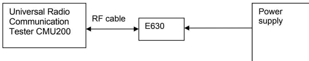
Figure 2. Test Set-up
