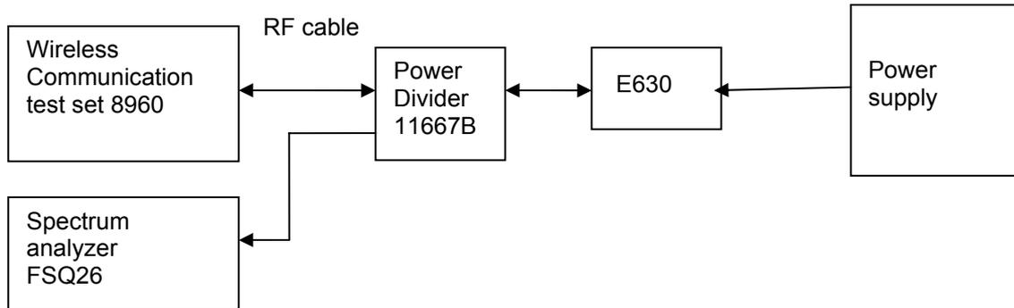
Figure 5. Test Set-up
