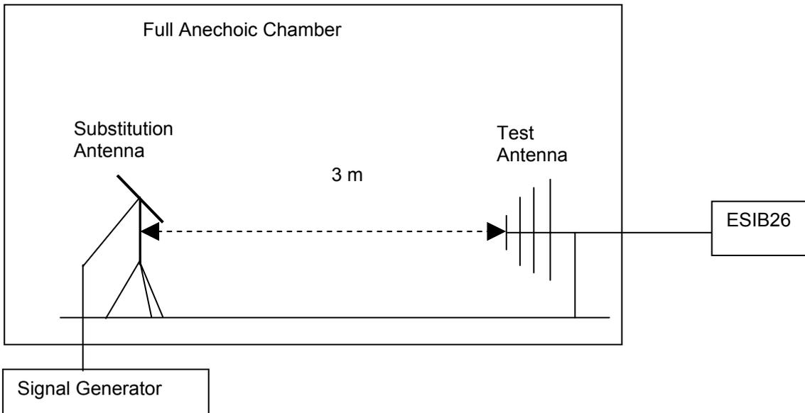
Figure 6. Test Set-up
