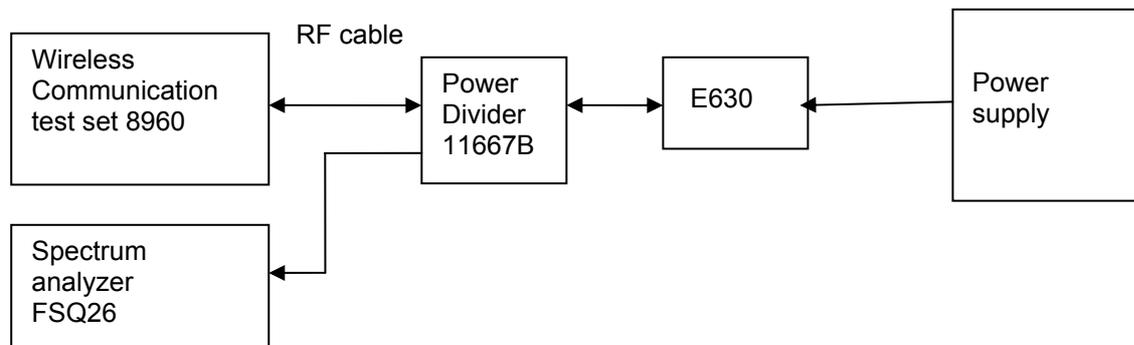
Figure 4. Test Set-up
