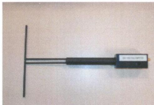
**Figure 1 – Satimo COMOSAR Validation Dipole**
