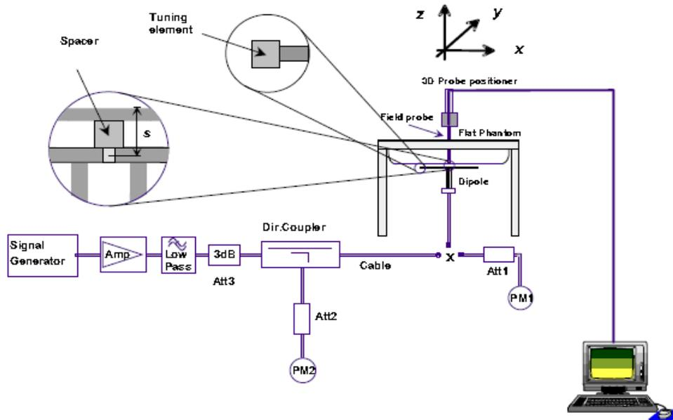
With the SG and Amp and with directional coupler in place, set up the source signal at the relevant frequency and use a power meter to measure the power at the end of the SMA cable that you intend to connect to the balanced dipole. Adjust the SG to make this, say, 0.25W (24 dBm). If this level is too high to read directly with the power meter sensor, insert a calibrated attenuator (e.g. 10 or 20 dB) and make a suitable correction to the power meter reading.
