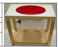
The ELI4 phantom is intended for compliance testing of handheld and body-mounted wireless devices in the frequency range of 30MHz to 6GHz. ELI4 is fully compatible with the latest draft of the standard IEC 62209-2 and all known tissue simulating liquids.
