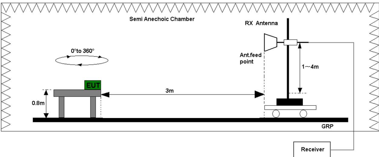
Figure 2. Test set-up of radiated disturbance(above 1GHz)
