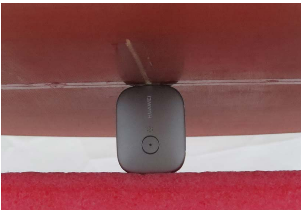
Picture 4: Right Side, the distance from handset to the bottom of the Phantom is 0mm
