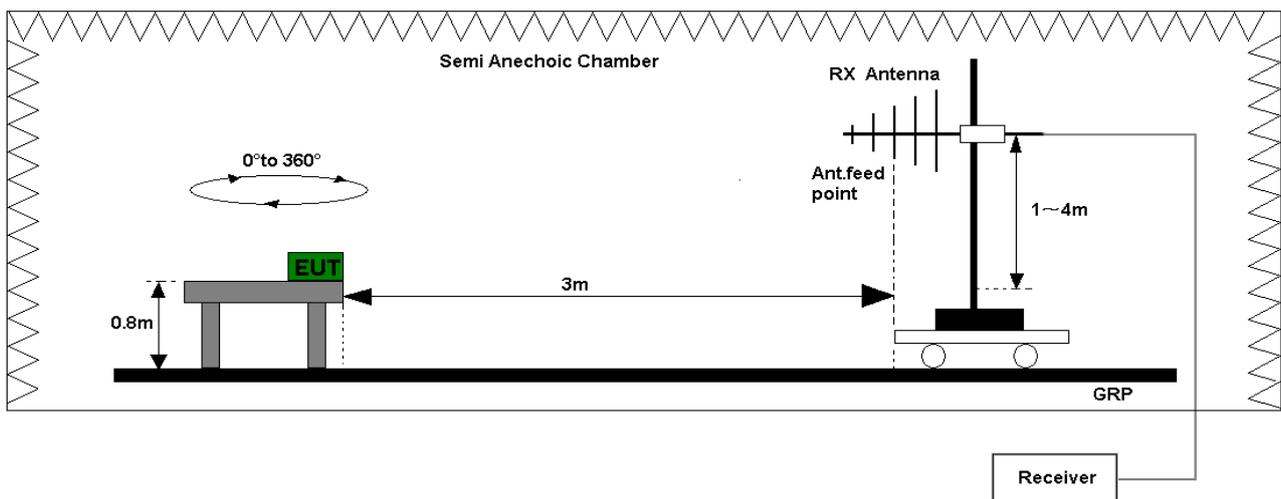
Figure 1. Test set-up of radiated disturbance(30MHz-1GHz )
