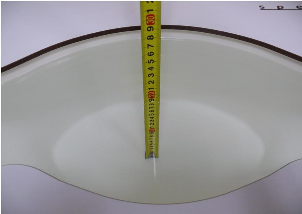
Picture 4 Liquid depth in the Flat Phantom (GSM1900)
