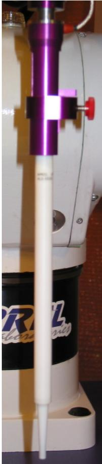
The April E-Field probe is evaluated to establish the diode compression point.
