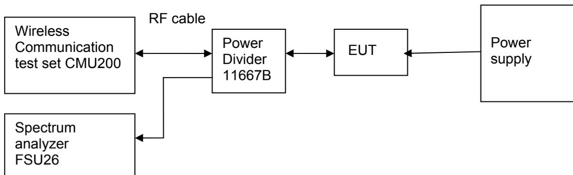
Figure 6. Test Set-up
