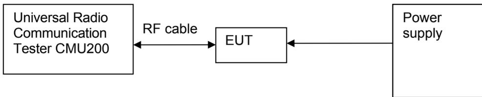
Figure 2. Test Set-up
