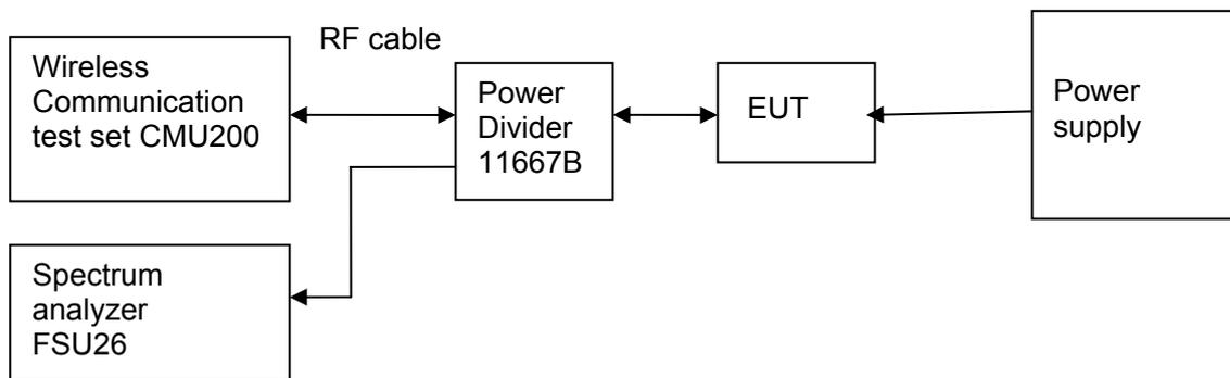
Figure 5. Test Set-up
