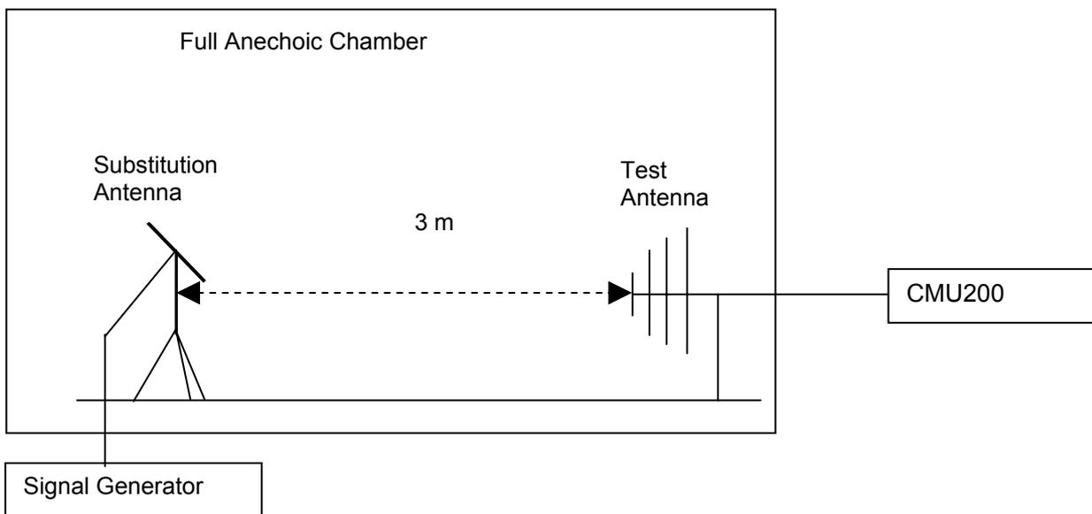
Figure 1. Test Set-up
