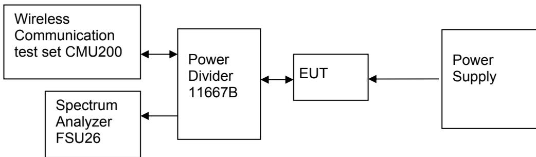
Figure 4. Test Set-up
