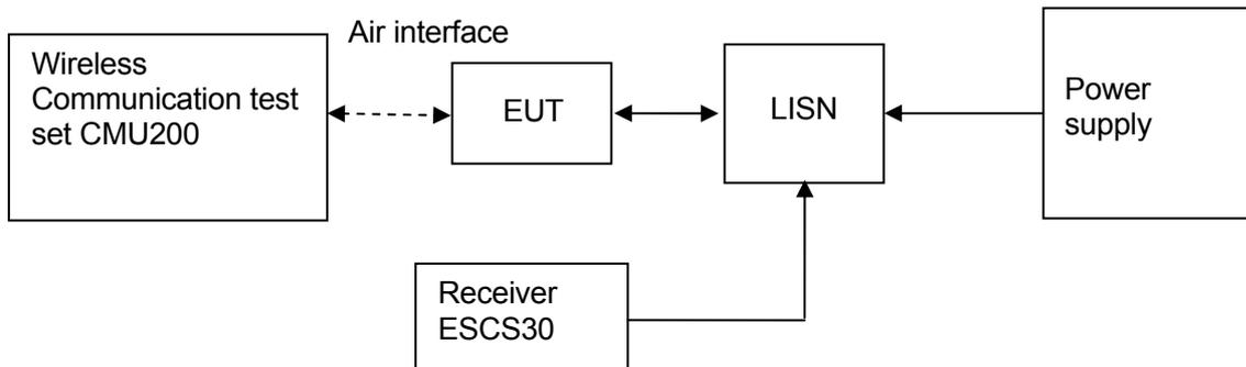
Figure 4. Test Set-up
