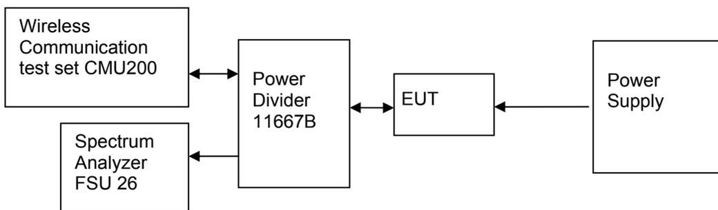
Figure 4. Test Set-up
