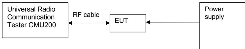
Figure 2. Test Set-up
