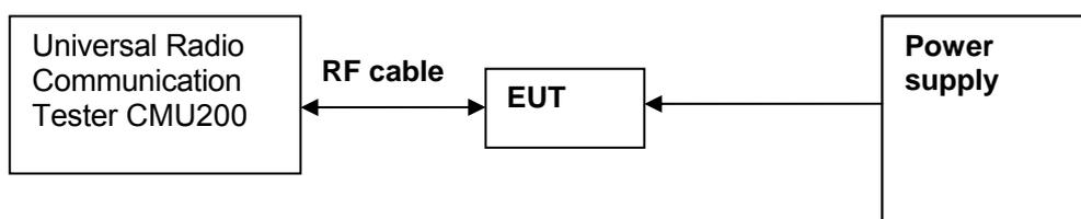
Figure 3. Test Set-up
