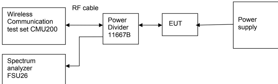
Figure 6. Test Set-up
