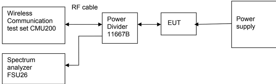
Figure 5. Test Set-up
