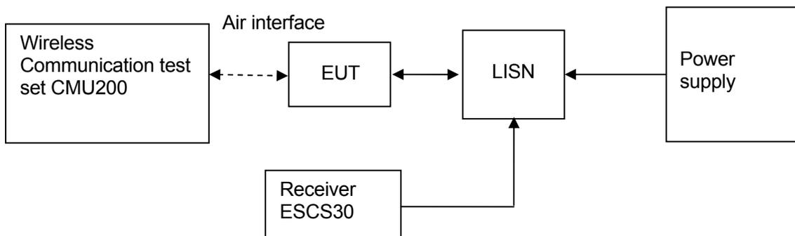
Figure 4. Test Set-up
