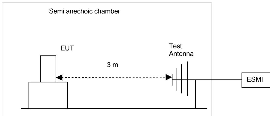
Figure 3. Test set-up
