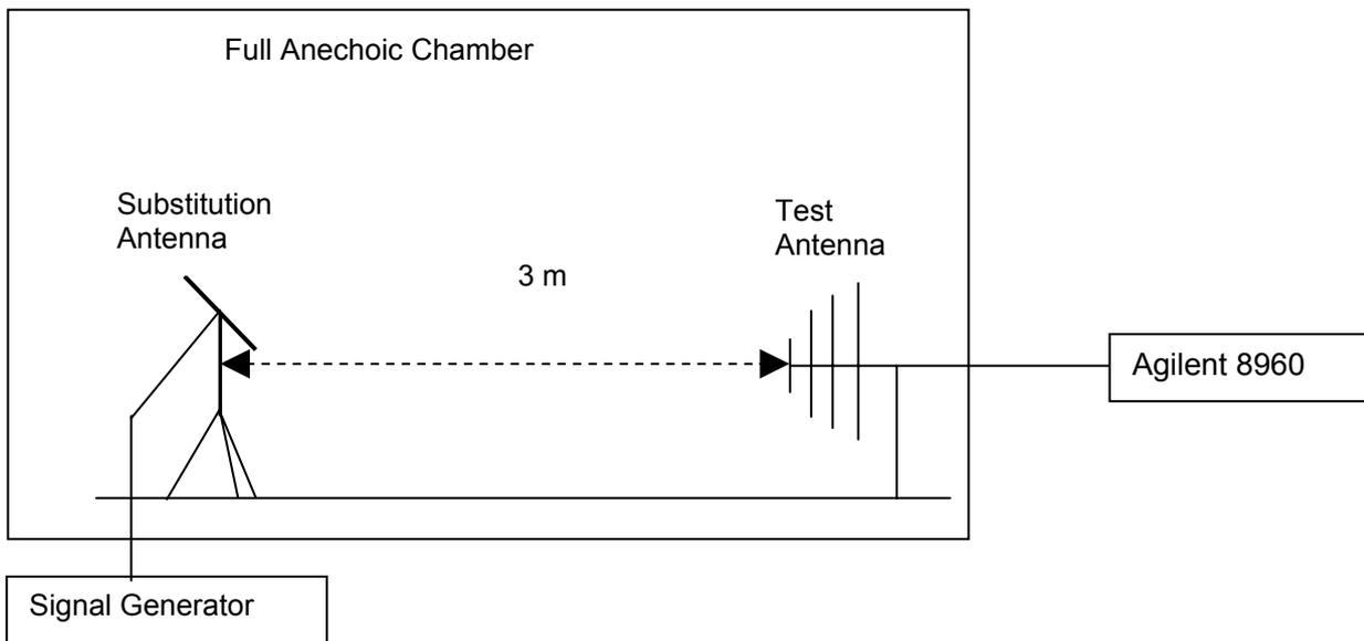
Figure 1. Test Set-up
