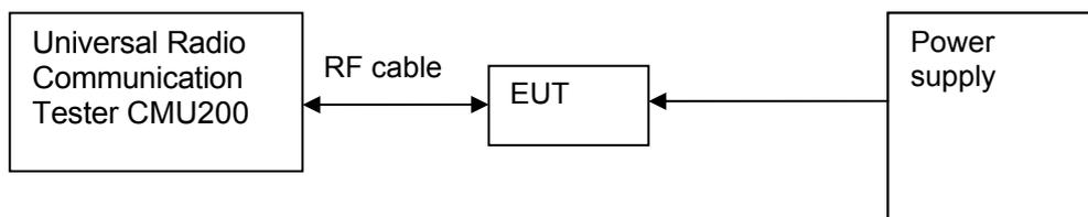
Figure 3. Test Set-up
