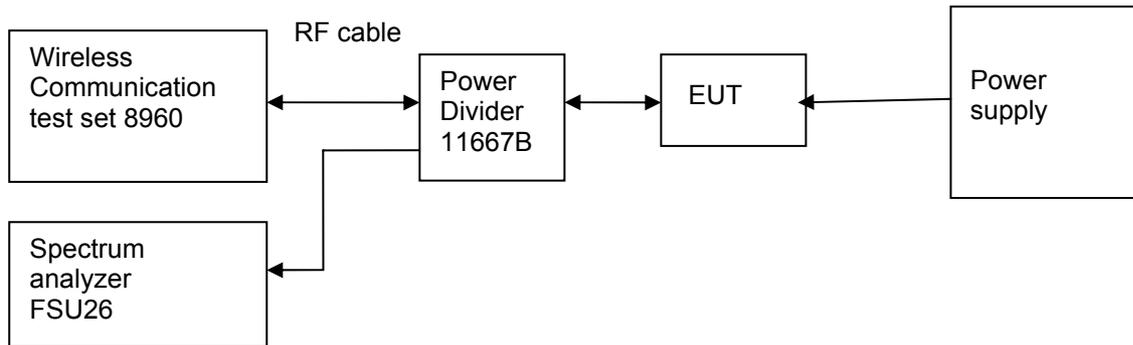
Figure 6. Test Set-up
