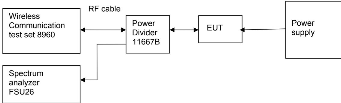
Figure 5. Test Set-up
