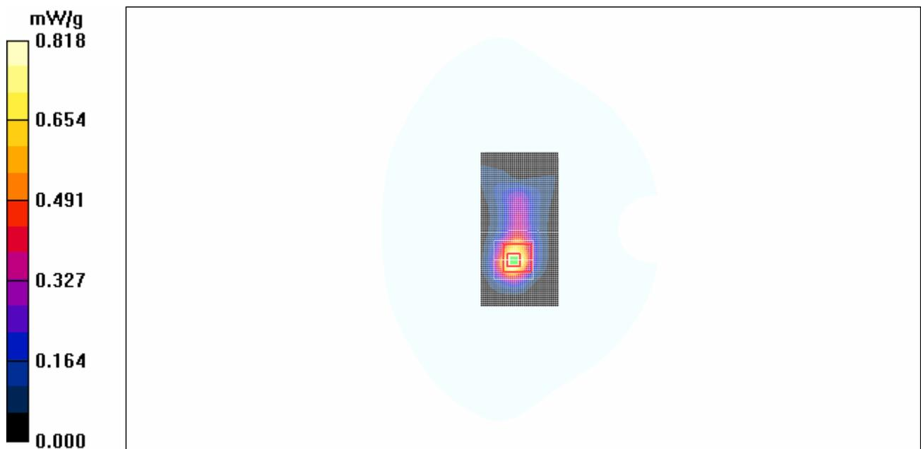
**Figure 25 GSM 1900 GPRS (3 timeslots in uplink) with BenQ Joy book S72 Test Position 1 Channel 661**
