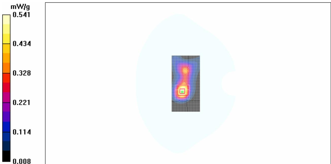
**Figure 29 GSM 1900 GPRS (1 timeslot in uplink) with BenQ Joy book S72 Test Position 1 Channel 661**
