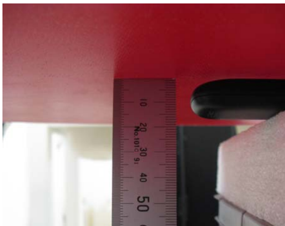
Picture 2-a: Test position 1 (EUT is connected to laptop via a USB cable which is shorter than 12 inches and distance between EUT and phantom is 5mm)
