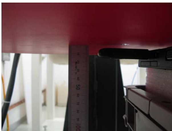
Picture 2-b: Test position 2 (distance between EUT and phantom is 5mm)
