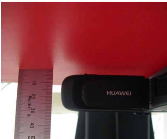
Picture 2-d: Test position 4 (distance between EUT and phantom is 5mm)
