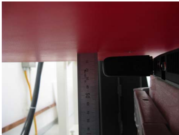
Picture 2-c: Test position 3 (distance between EUT and phantom is 5mm)
