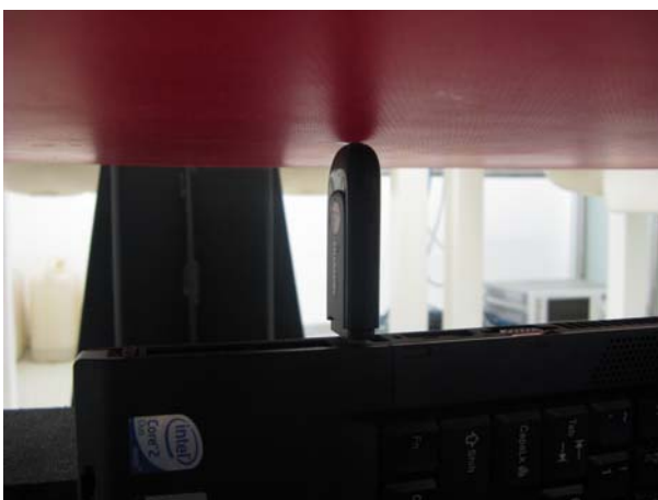
Picture 2-e: Test position 5 (distance between EUT and phantom is 0mm)
