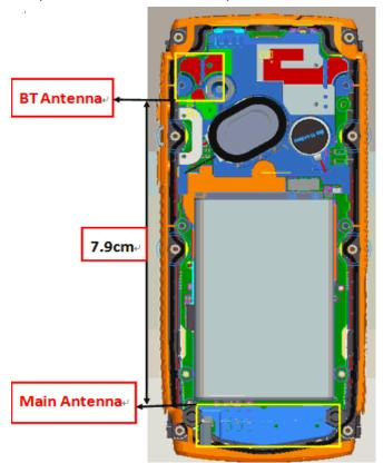
The output power of BT antenna is as following:
