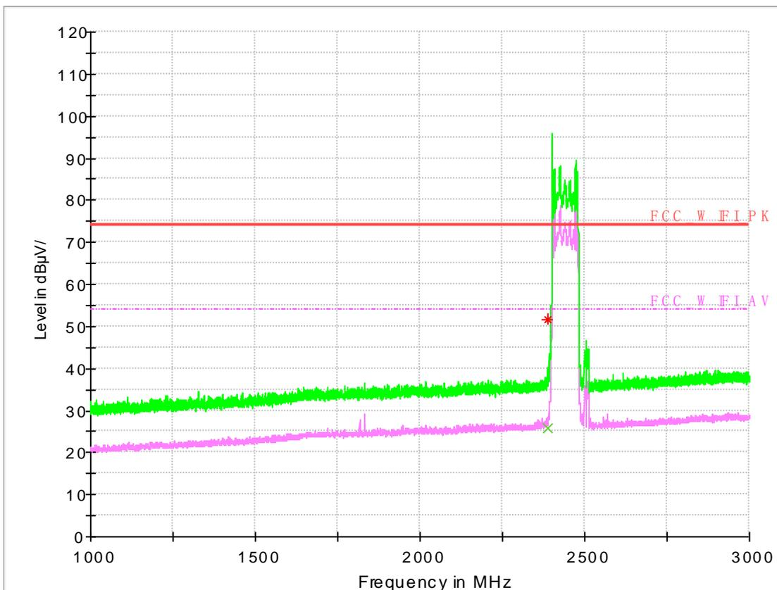
**Note: The peak exceeds the limit line is carrier frequency.**
