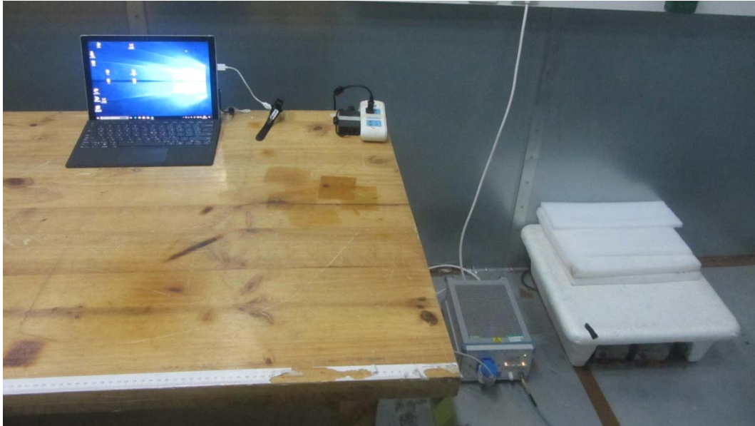
Picture 2 Conducted Emission Test Setup
