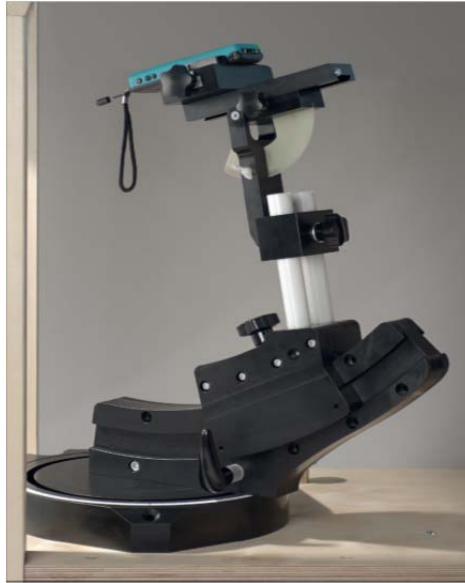
F-2. Device Holder for Transmitters
