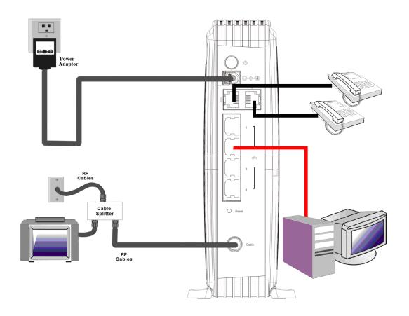
Fig. How to set up your connection
