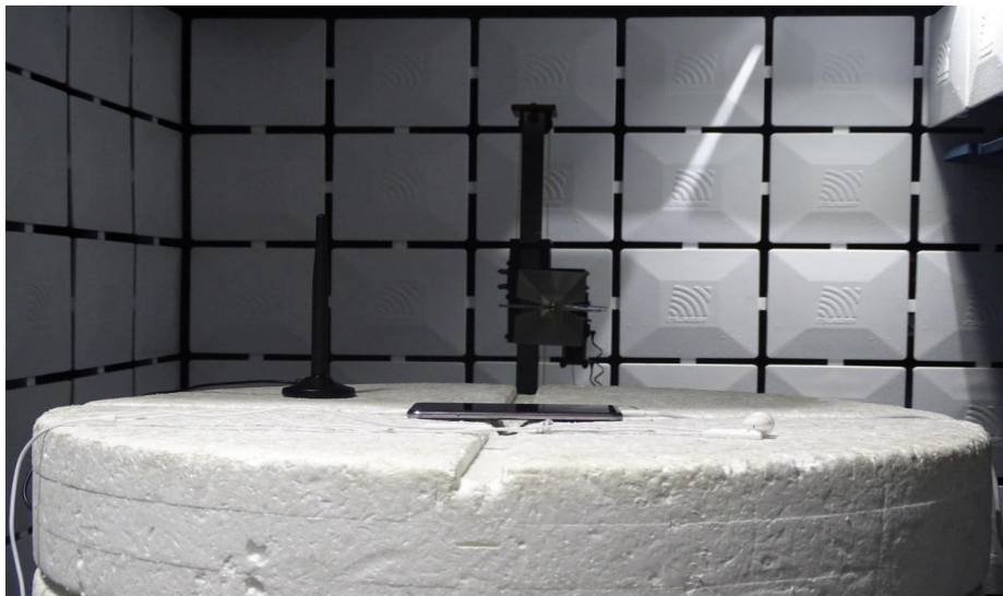
Radiated Spurious Emission (3GHz to 18GHz)
