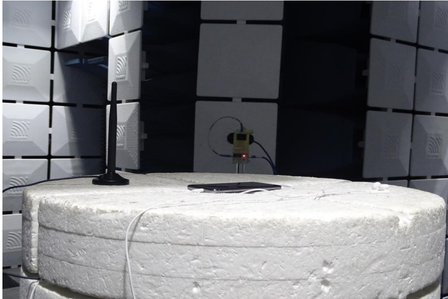
Radiated Spurious Emission (18GHz to26.5GHz)
