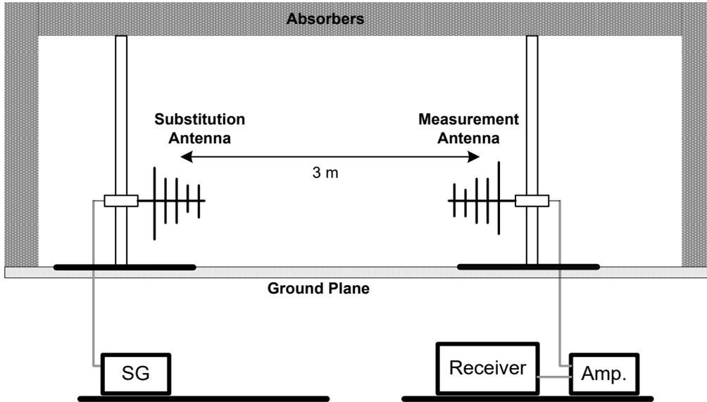
**Above 1GHz- Substitution method to verify the maximum ERP/EIRP**
