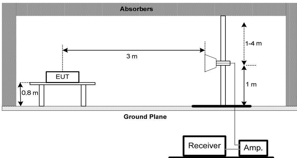
**30MHz to 1GHz- Substitution method to verify the maximum ERP/EIRP**
