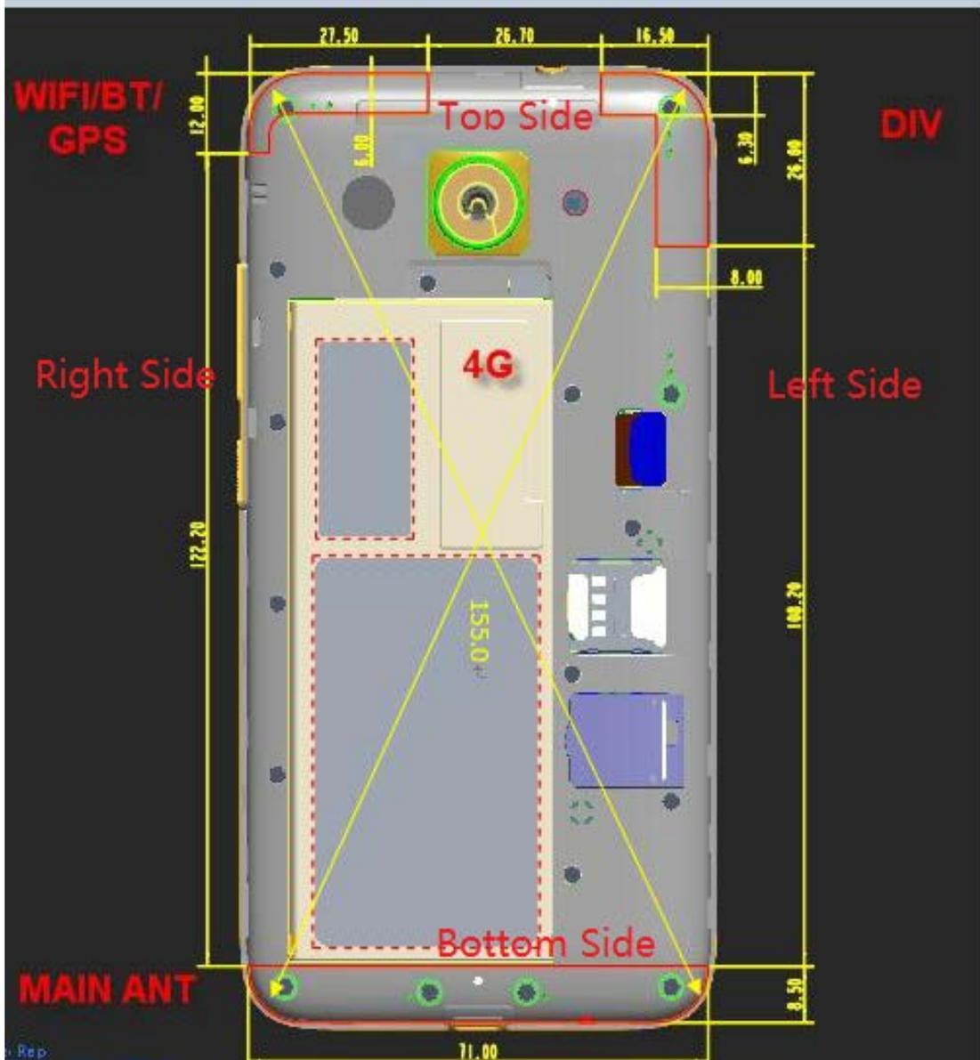
Note: The Div antenna is used to improve the acceptance of performance of the main antenna, it does not have a transmitter function.
