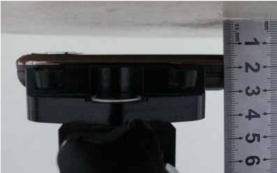
Picture 10: Body, towards phantom, the distance from handset to the bottom of the Phantom is 15mm)
