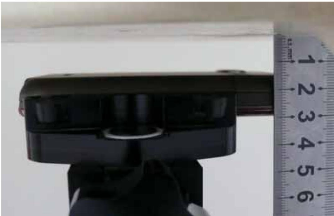
Picture 9: Body, The EUT display towards ground, the distance from handset to the bottom of the Phantom is 15mm)
