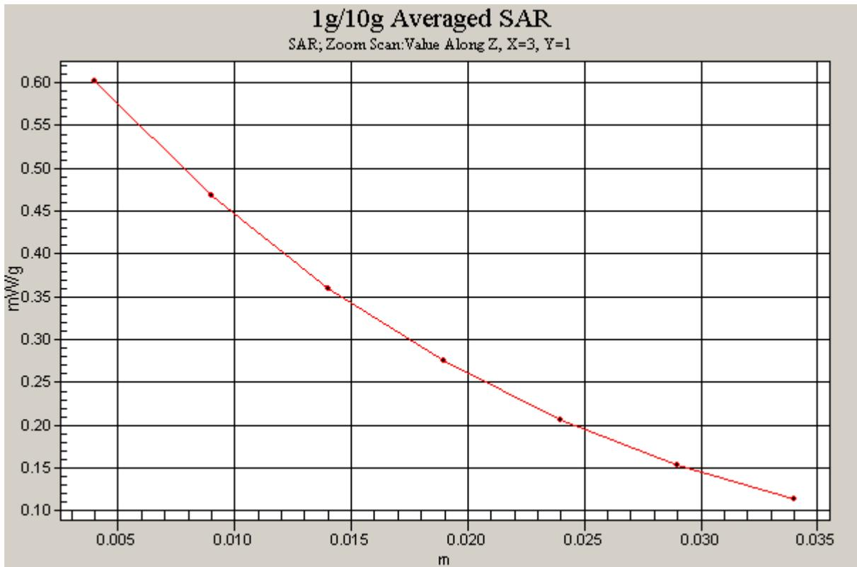
Figure 17 Z-Scan at power reference point (Left Hand Tilt 15° CDMA Cellular Channel 384)
