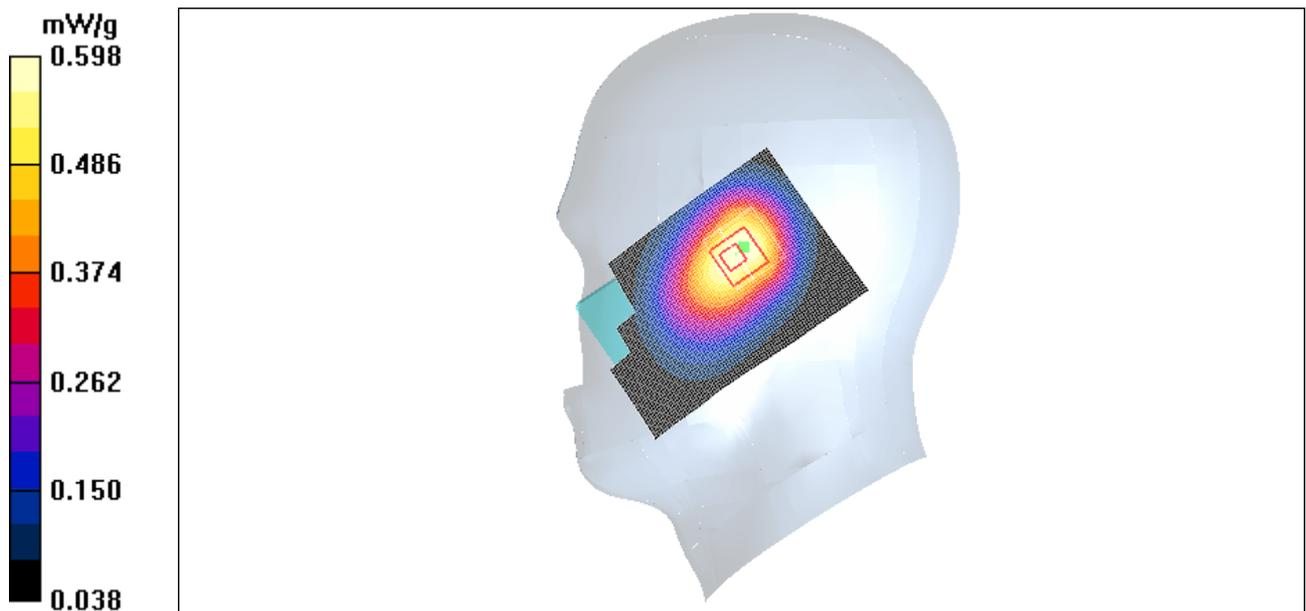
Figure 30 Right Hand Tilt 15° CDMA Cellular Channel 1013
