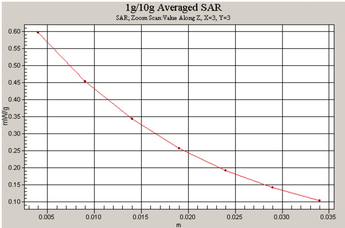
Figure 29 Z-Scan at power reference point (Right Hand Tilt 15° CDMA Cellular Channel 384)
