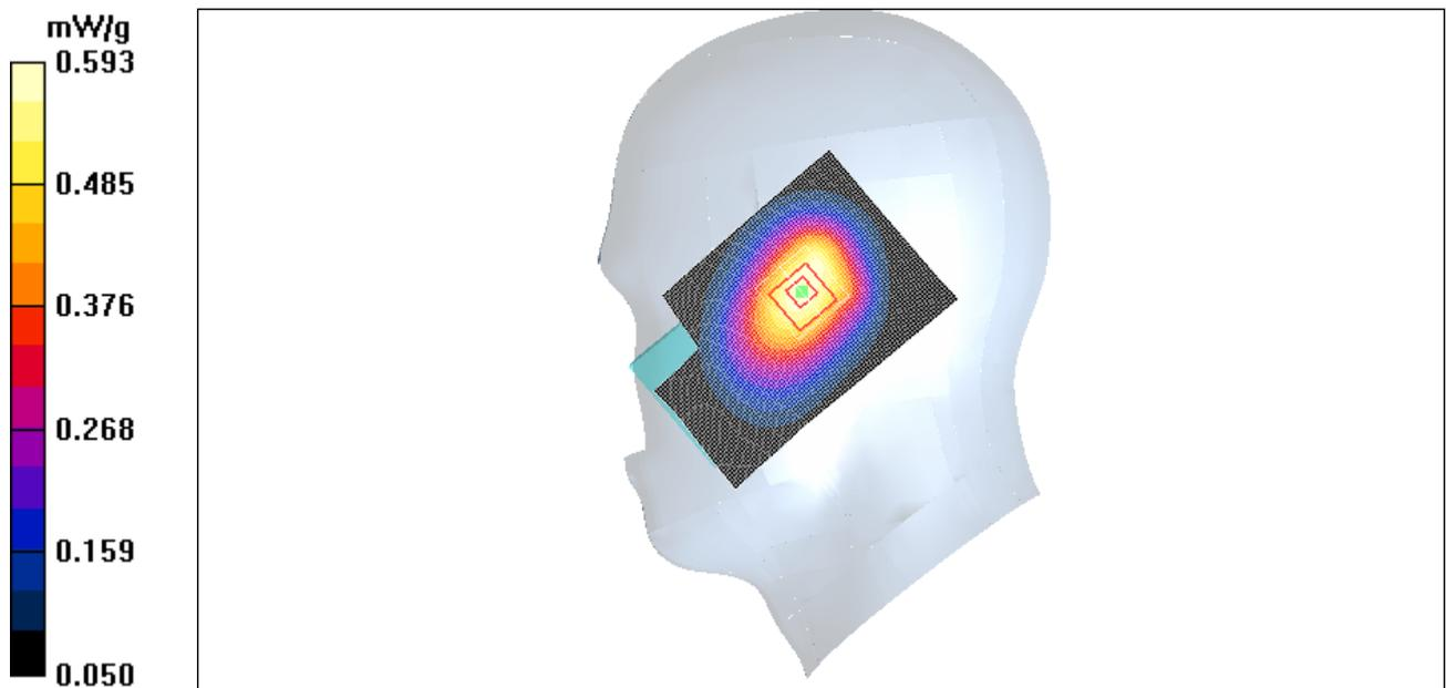
Figure 28 Right Hand Tilt 15° CDMA Cellular Channel 384
