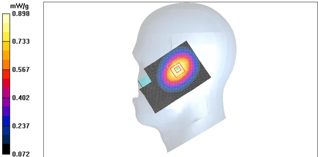
Figure 24 Right Hand Touch Cheek CDMA Cellular Channel 1013
