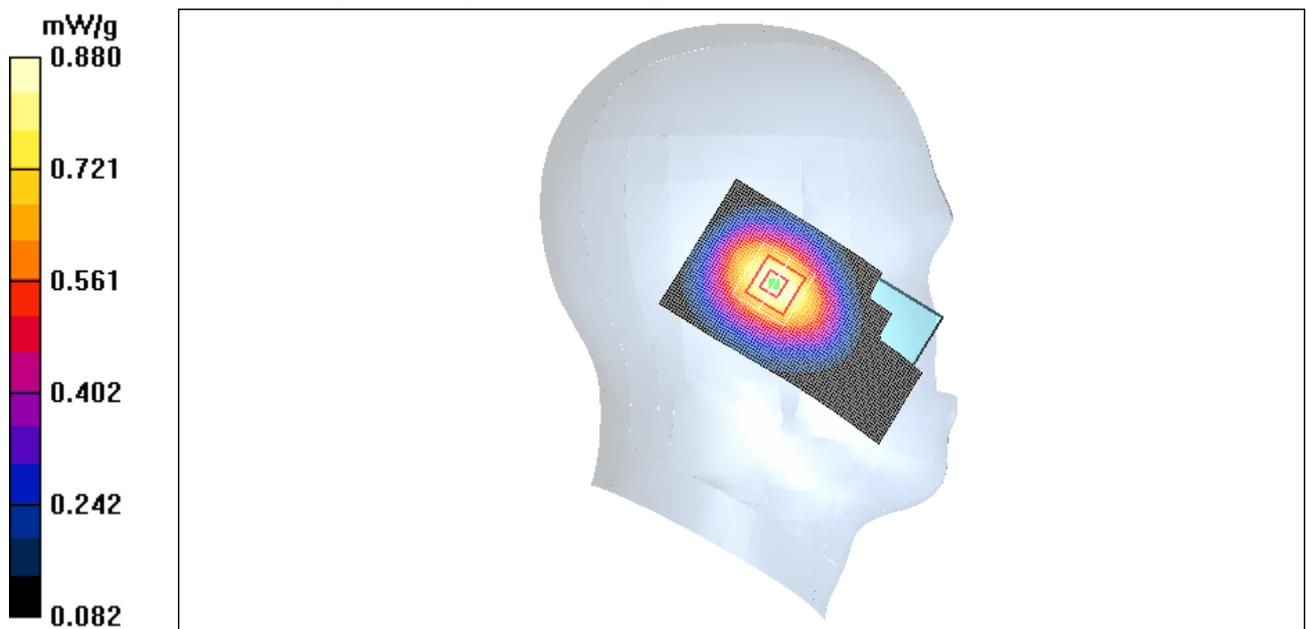
Figure 10 Left Hand Touch Cheek CDMA Cellular Channel 384
