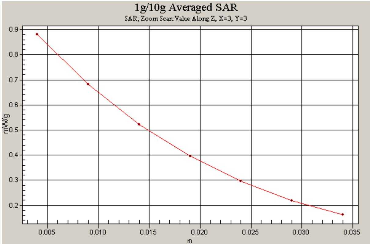
Figure 11 Z-Scan at power reference point (Left Hand Touch Cheek CDMA Cellular Channel 384)
