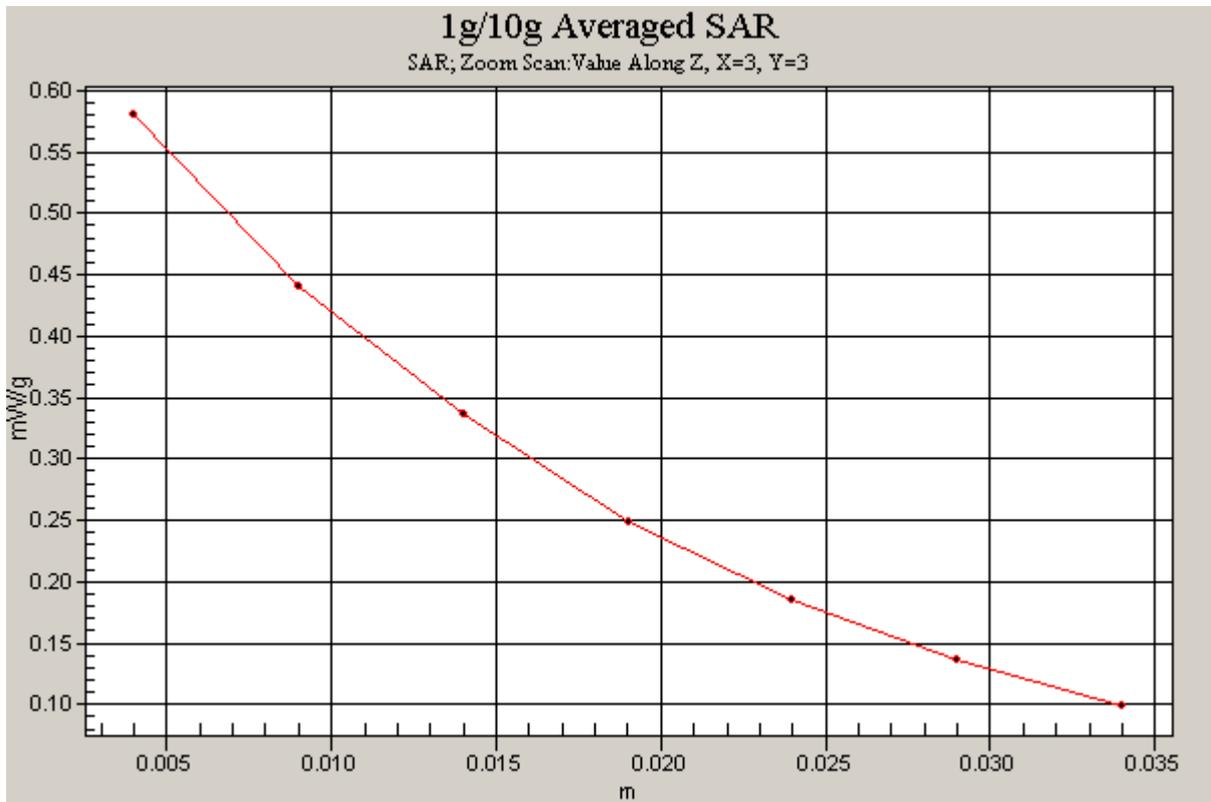
Figure 27 Z-Scan at power reference point (Right Hand Tilt 15° CDMA Cellular Channel 777)
