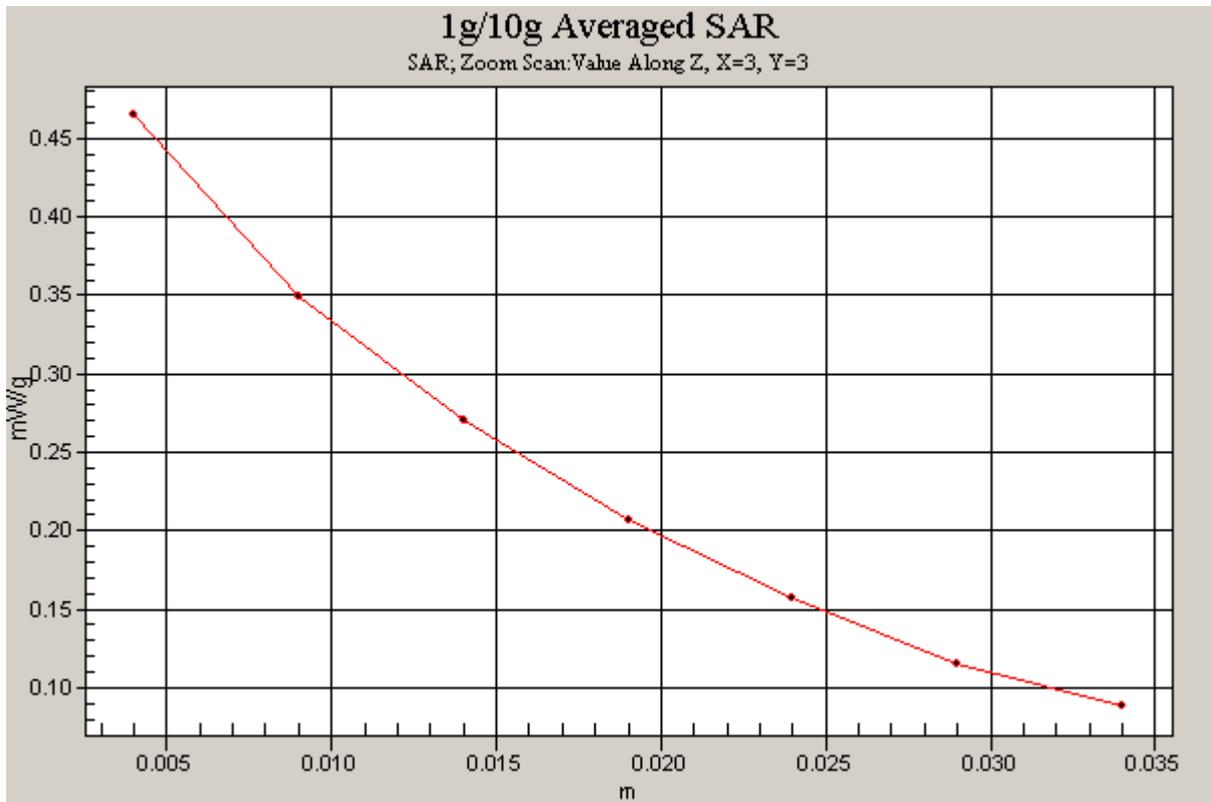
Figure 39 Z-Scan at power reference point (Body, Towards Phantom, CDMA Cellular Channel 777)
