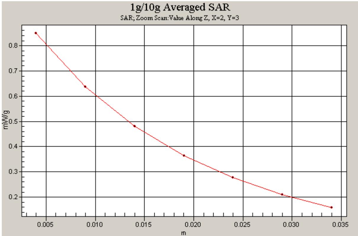
Figure 33 Z-Scan at power reference point (Body, Towards Ground, CDMA Cellular Channel 777)
