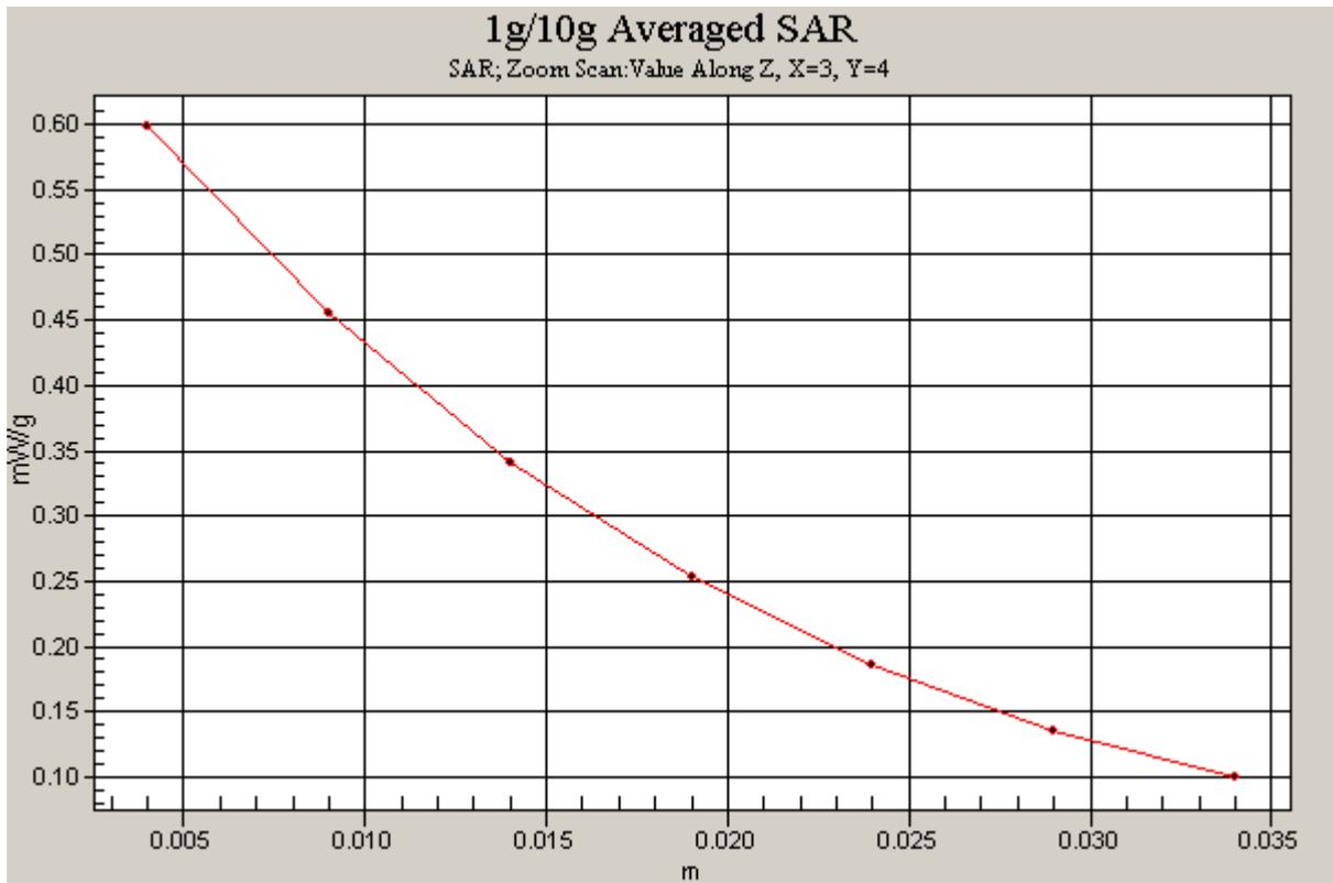
Figure 31 Z-Scan at power reference point (Right Hand Tilt 15° CDMA Cellular Channel 1013)
