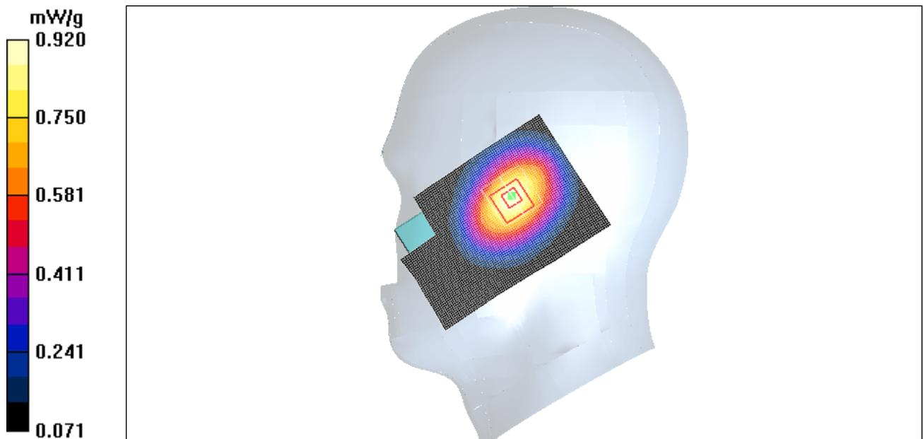
Figure 20 Right Hand Touch Cheek CDMA Cellular Channel 777
