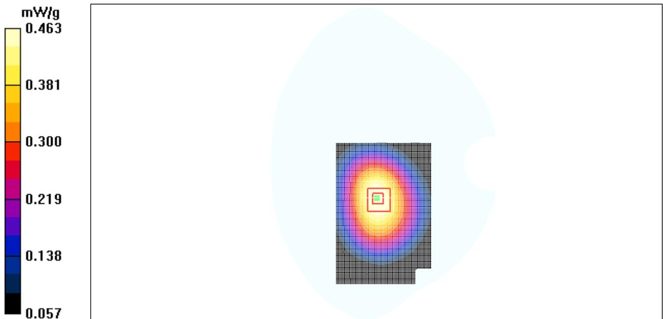
Figure 38 Body, Towards Phantom, CDMA Cellular Channel 777
