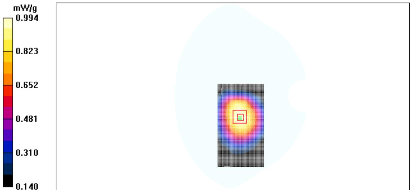
Figure 36 Body, Towards Ground, CDMA Cellular Channel 1013
