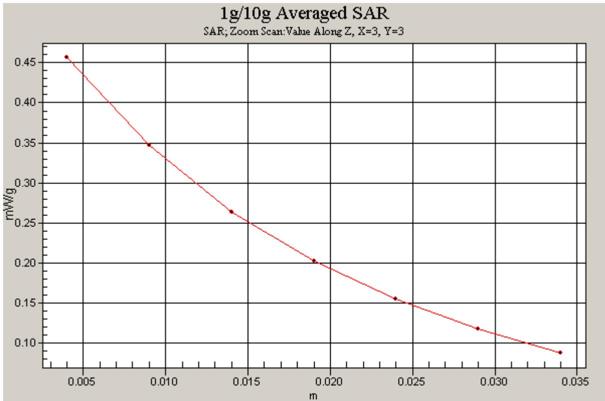
Figure 41 Z-Scan at power reference point (Body, Towards Phantom, CDMA Cellular Channel 384)
