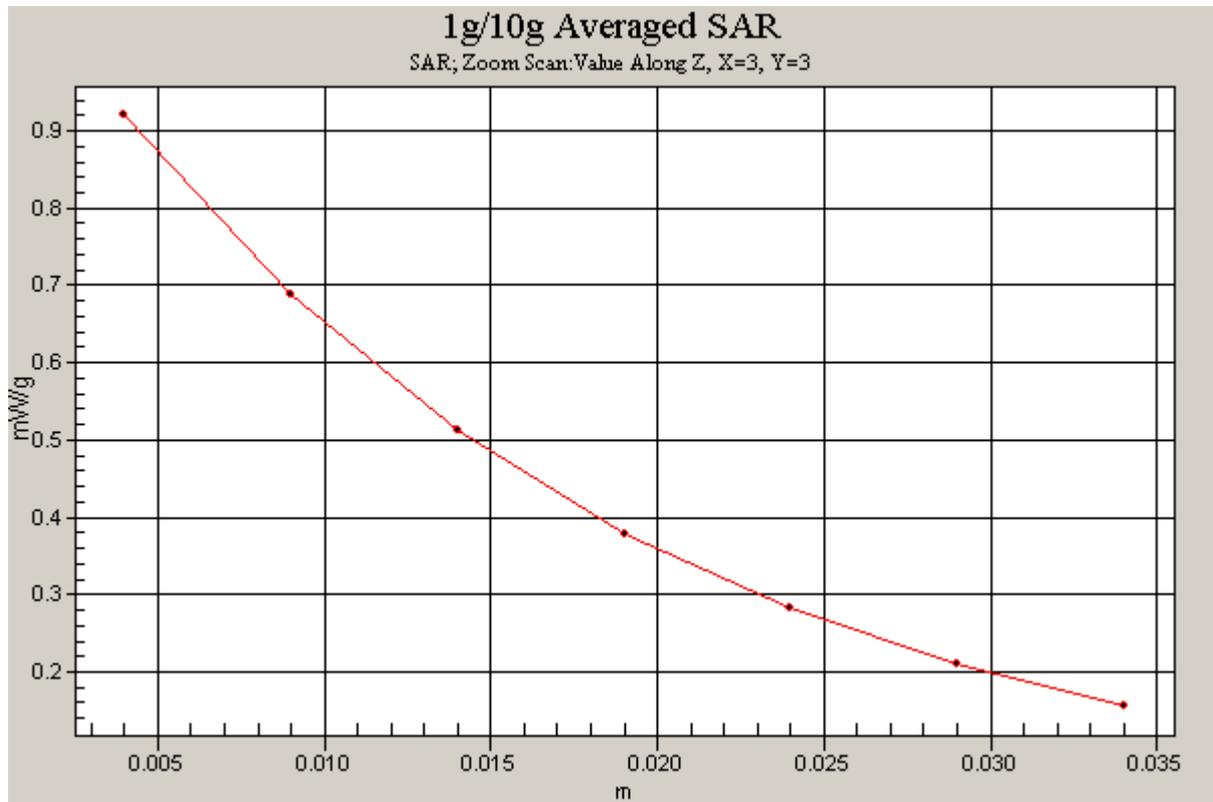
Figure 21 Z-Scan at power reference point (Right Hand Touch Cheek CDMA Cellular Channel 777)
