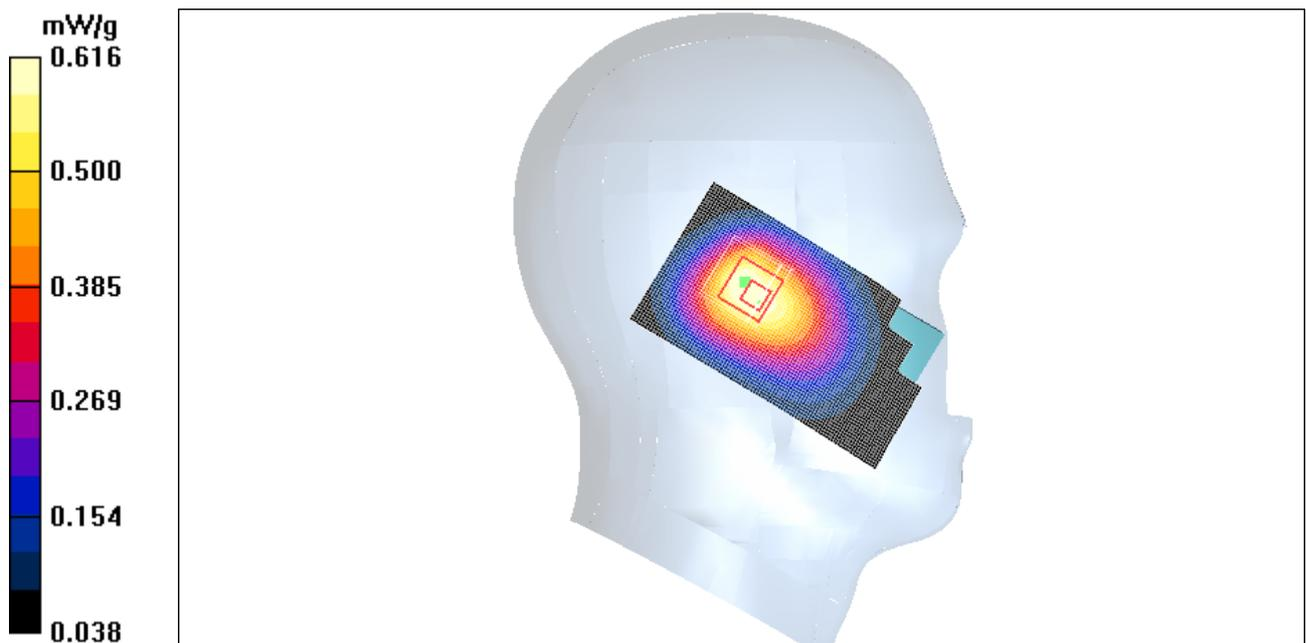
Figure 14 Left Hand Tilt 15° CDMA Cellular Channel 777
