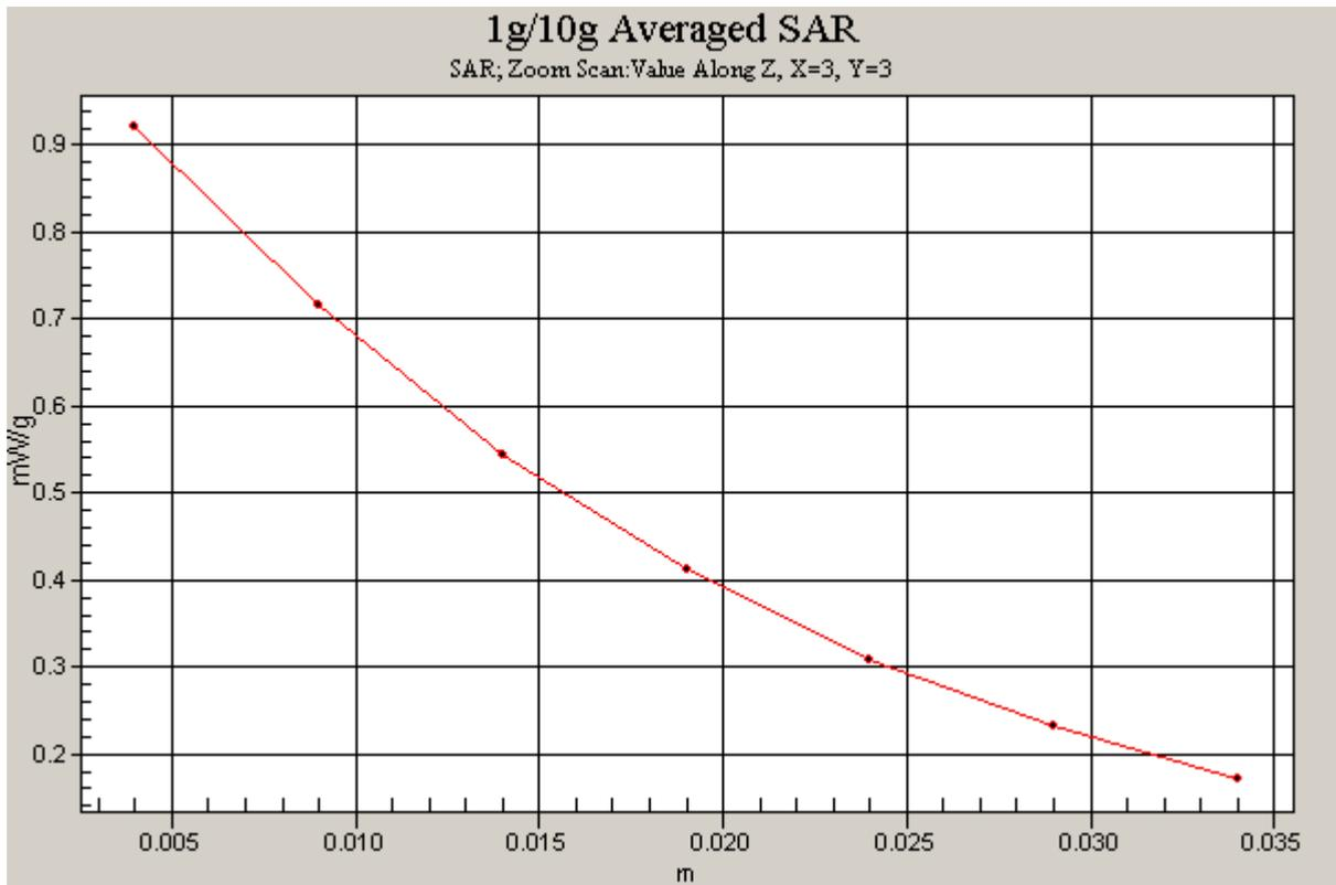
Figure 13 Z-Scan at power reference point (Left Hand Touch Cheek CDMA Cellular Channel 1013)
