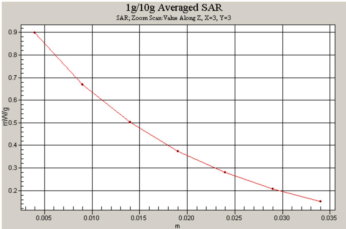
Figure 25 Z-Scan at power reference point (Right Hand Touch Cheek CDMA Cellular Channel 1013)
