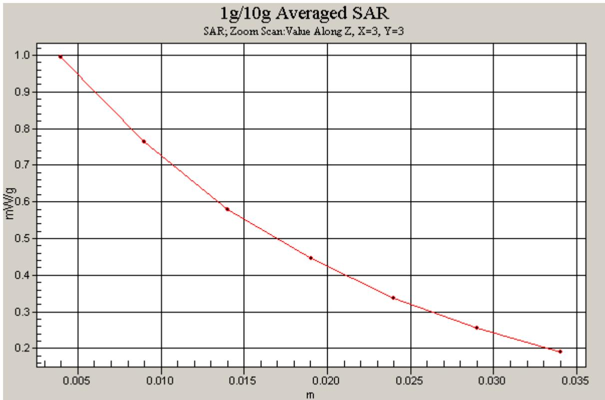
Figure 37 Z-Scan at power reference point (Body, Towards Ground, CDMA Cellular Channel 1013)
