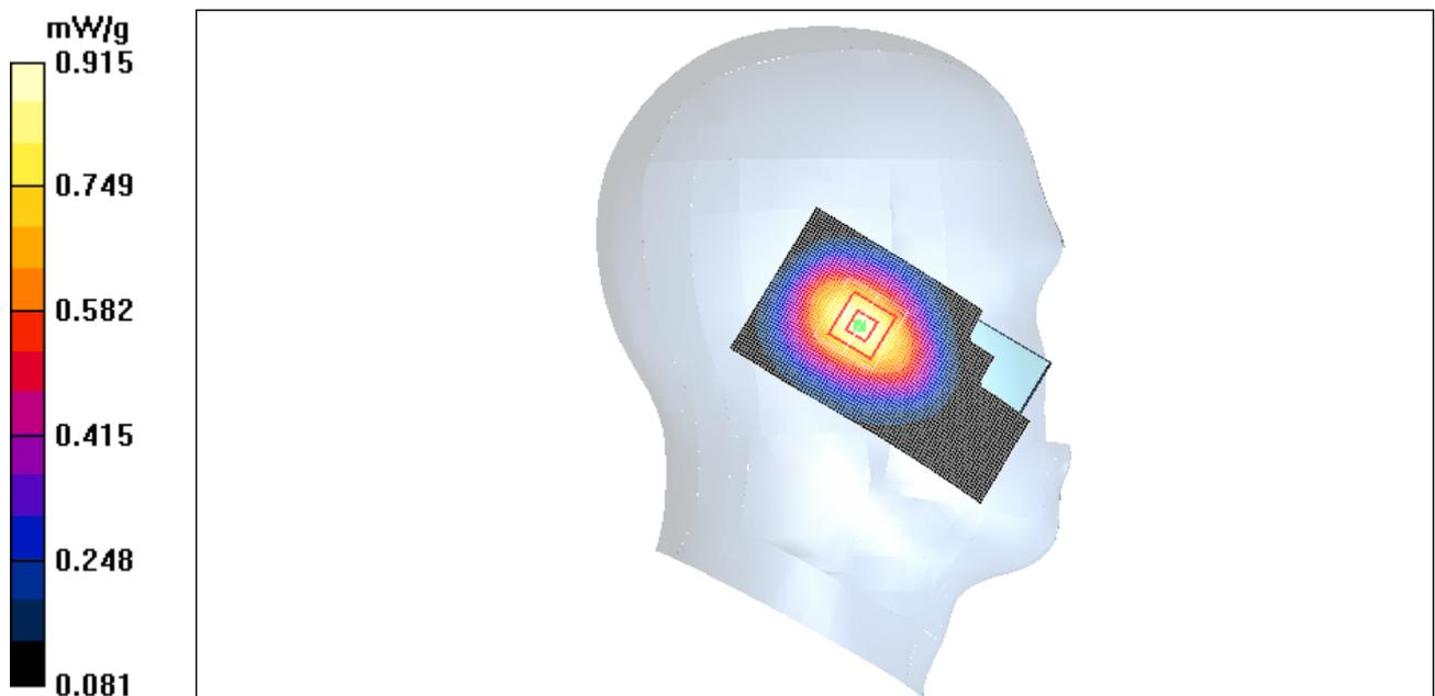
Figure 8 Left Hand Touch Cheek CDMA Cellular Channel 777
