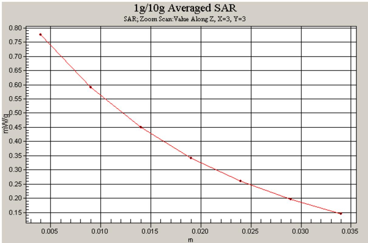
**Figure 45 Z-Scan at power reference point (Body with earphone, Towards Ground, CDMA Cellular Channel 1013)**
