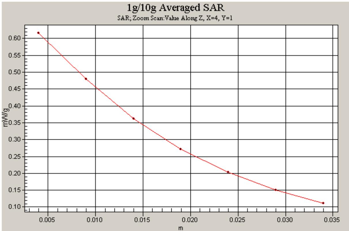
Figure 15 Z-Scan at power reference point (Left Hand Tilt 15° CDMA Cellular Channel 777)
