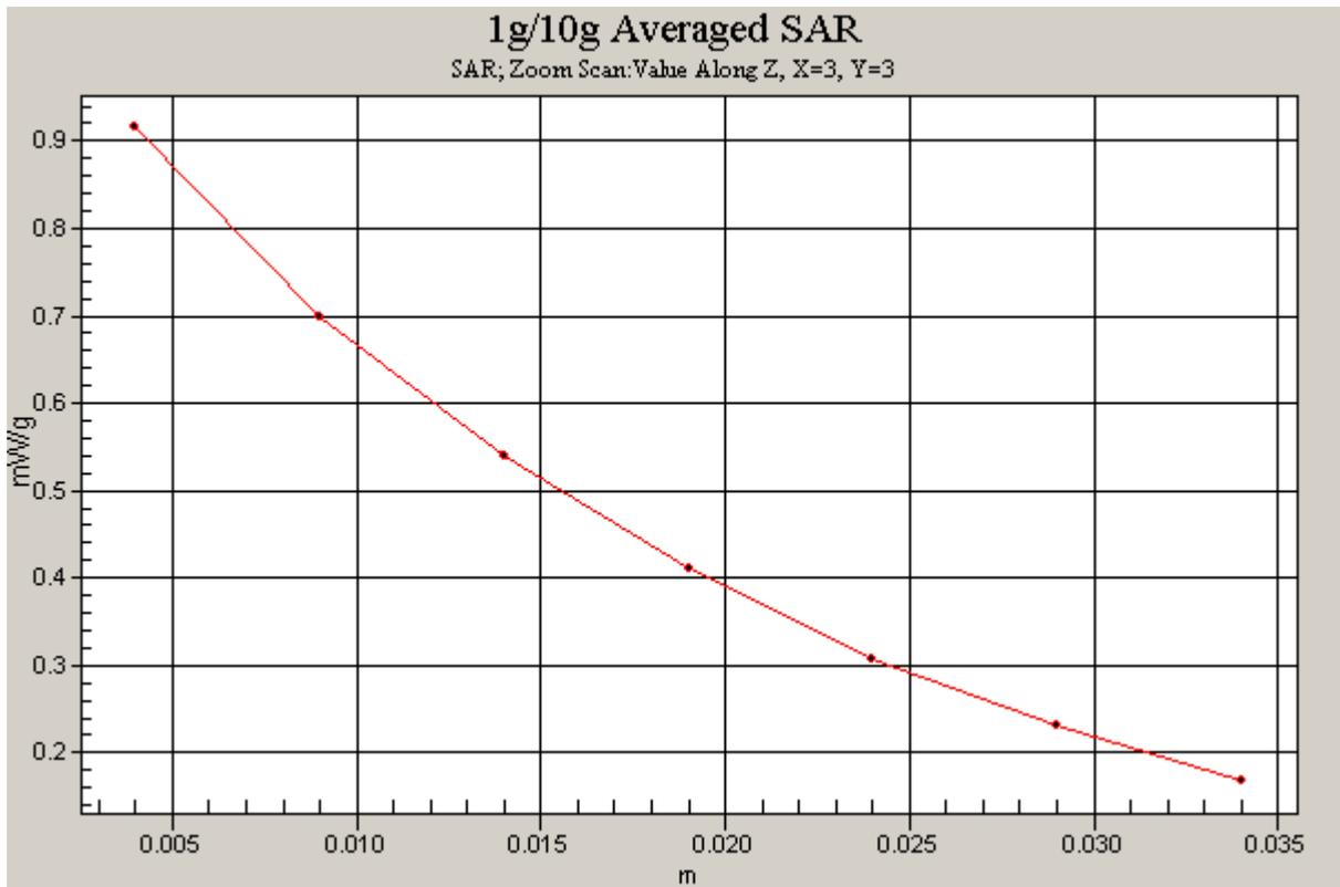
Figure 9 Z-Scan at power reference point (Left Hand Touch Cheek CDMA Cellular Channel 777)
