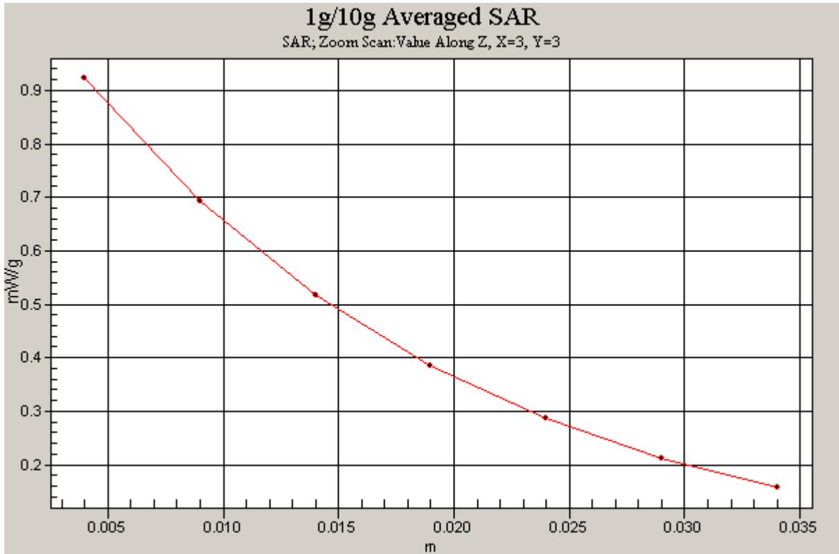
Figure 23 Z-Scan at power reference point (Right Hand Touch Cheek CDMA Cellular Channel 384)
