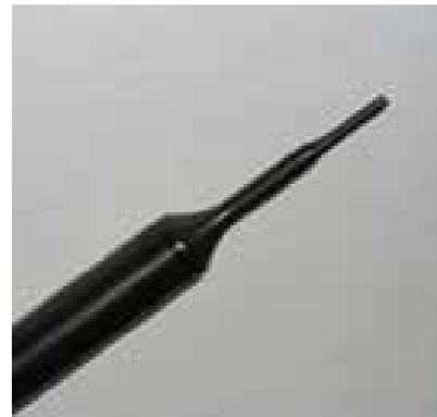
Figure 2. EX3DV4 E-field Probe
