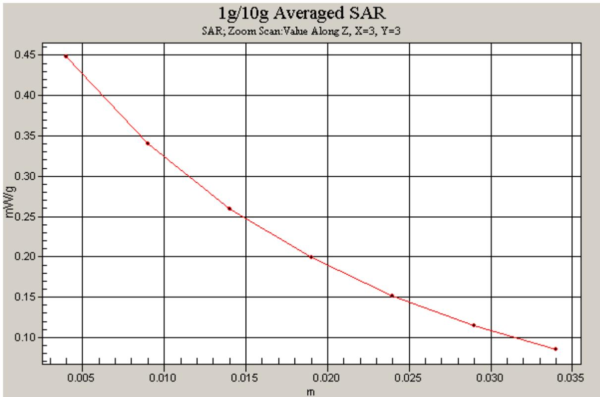
Figure 43 Z-Scan at power reference point (Body, Towards Phantom, CDMA Cellular Channel 1013)
