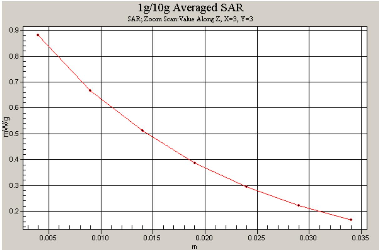
Figure 35 Z-Scan at power reference point (Body, Towards Ground, CDMA Cellular Channel 384)
