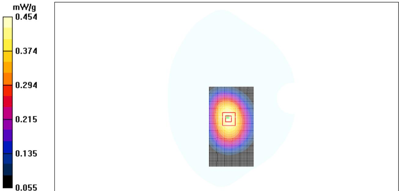
Figure 40 Body, Towards Phantom, CDMA Cellular Channel 384
