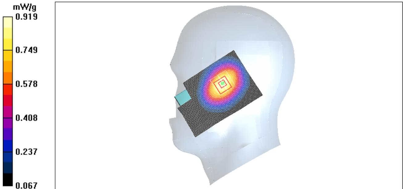
Figure 22 Right Hand Touch Cheek CDMA Cellular Channel 384
