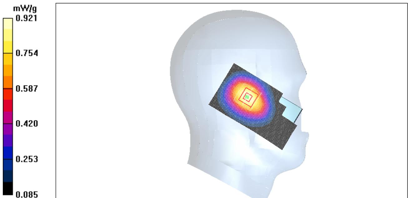
Figure 12 Left Hand Touch Cheek CDMA Cellular Channel 1013
