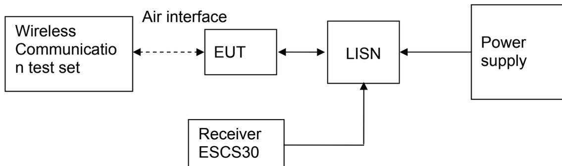
Figure 3. Test Set-up
