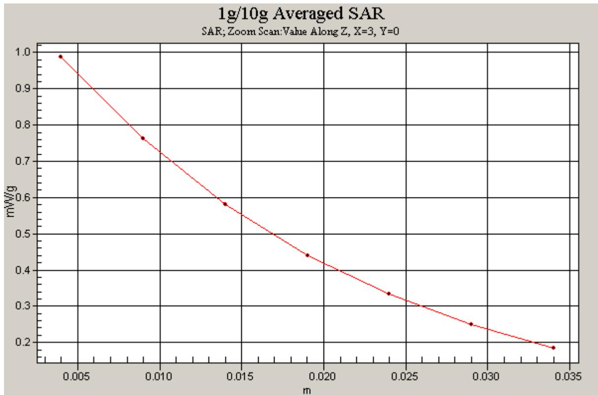
Figure 28 Z-Scan at power reference point (Body, Towards Ground, CDMA Cellular Channel 1013)
