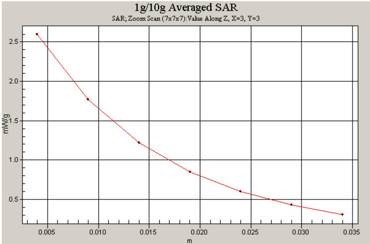
Figure 10 Z-Scan at power reference point (System Check at 835 MHz Dipole)
