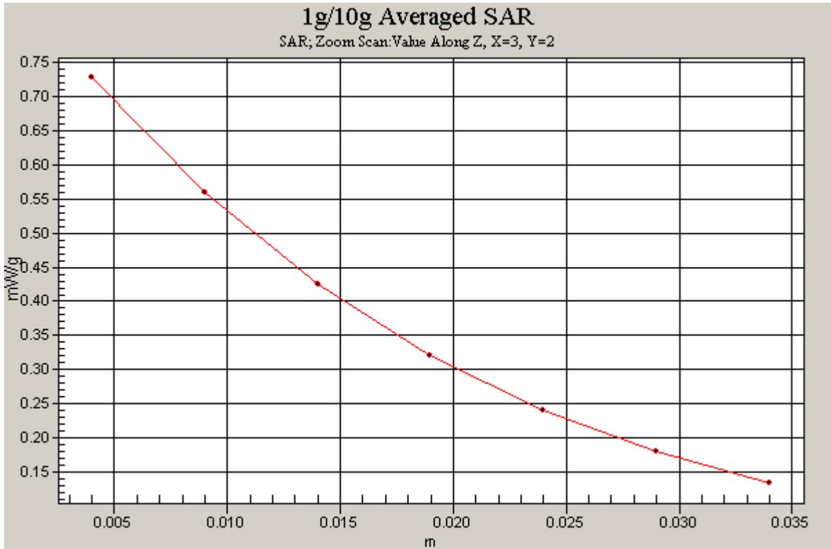
Figure 12 Z-Scan at power reference point (Left Hand Touch Cheek CDMA Cellular Channel 777)
