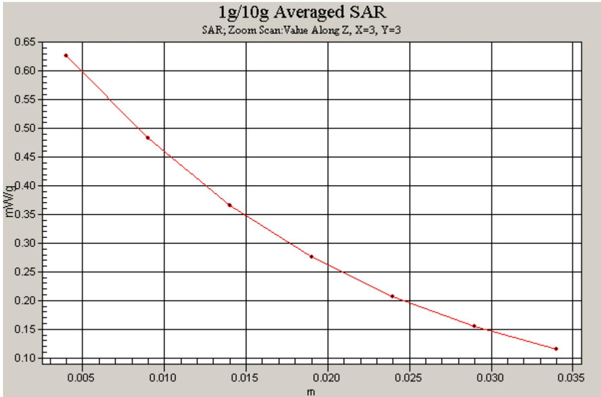
Figure 14 Z-Scan at power reference point (Left Hand Touch Cheek CDMA Cellular Channel 384)
