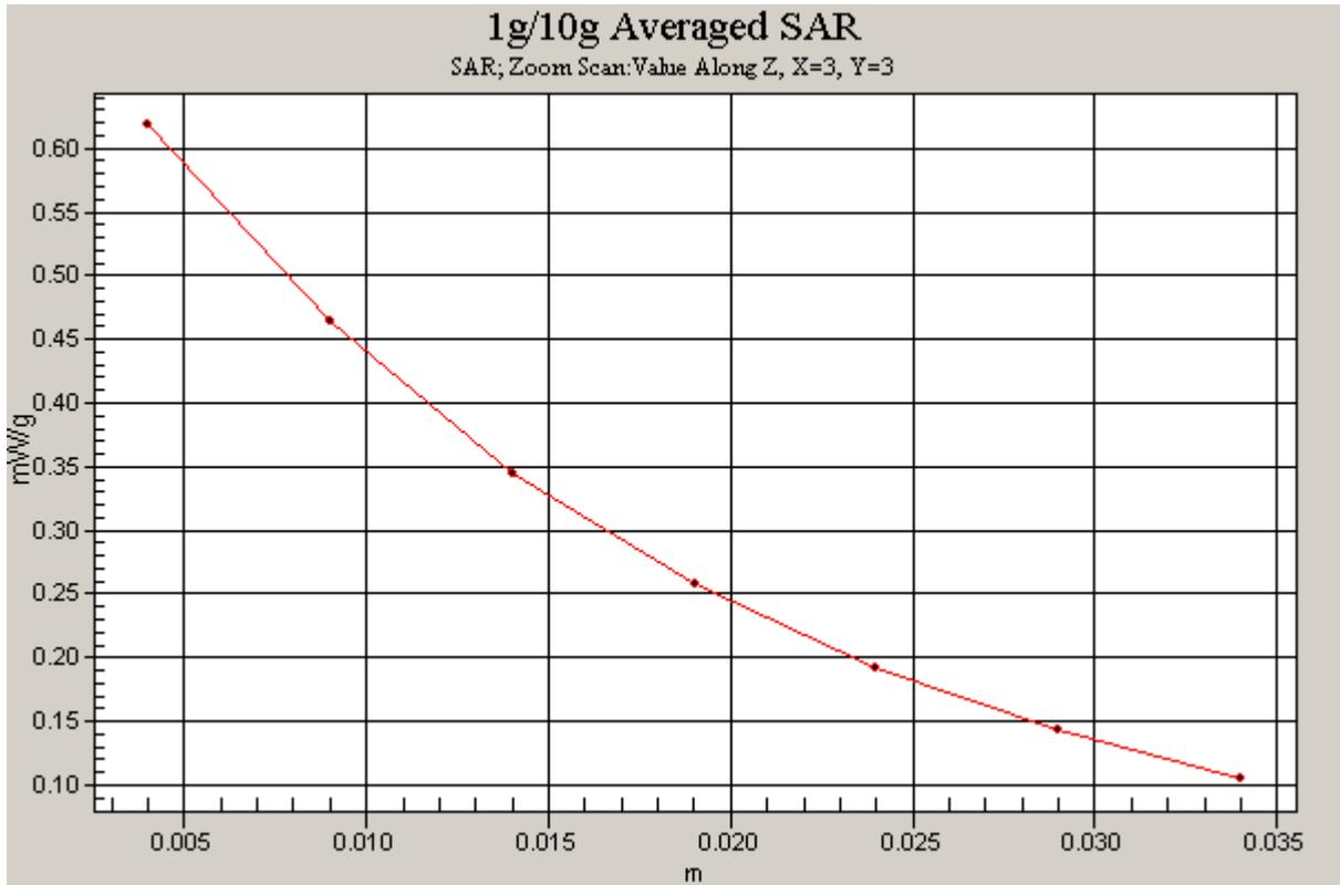
Figure 20 Z-Scan at power reference point (Right Hand Touch Cheek CDMA Cellular Channel 384)
