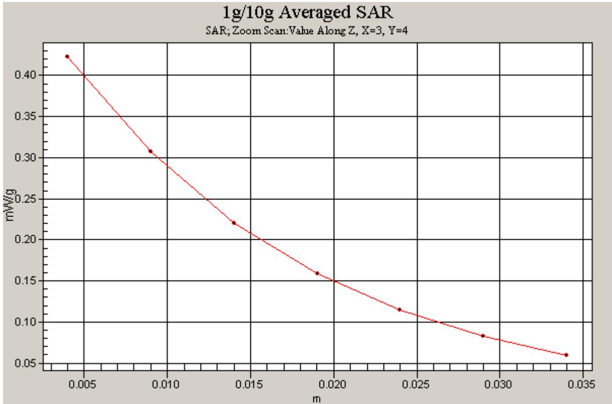
Figure 22 Z-Scan at power reference point (Right Hand Tilt 15° CDMA Cellular Channel 384)
