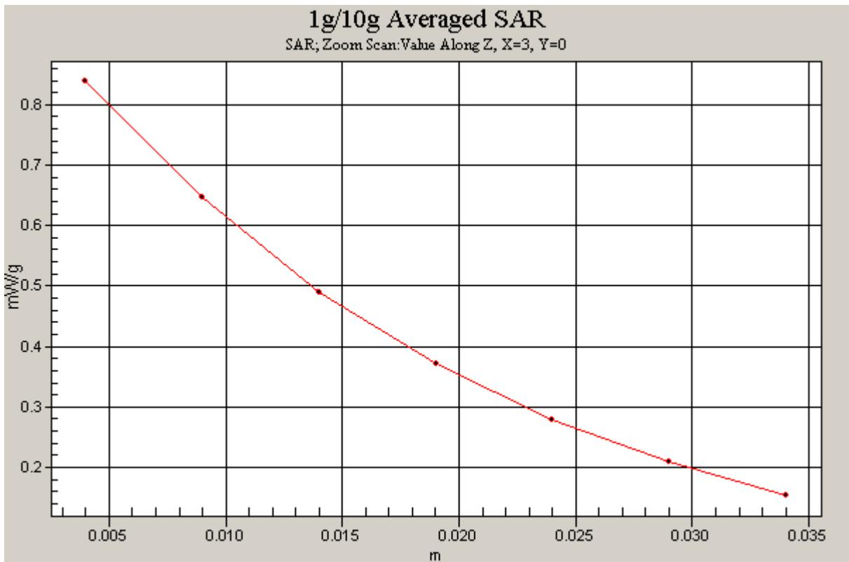
Figure 24 Z-Scan at power reference point (Body, Towards Ground, CDMA Cellular Channel 777)
