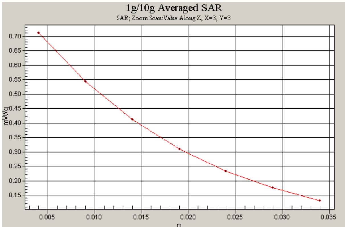
Figure 32 Z-Scan at power reference point (Body with Earphone, Towards Ground, CDMA Cellular Channel 384)
