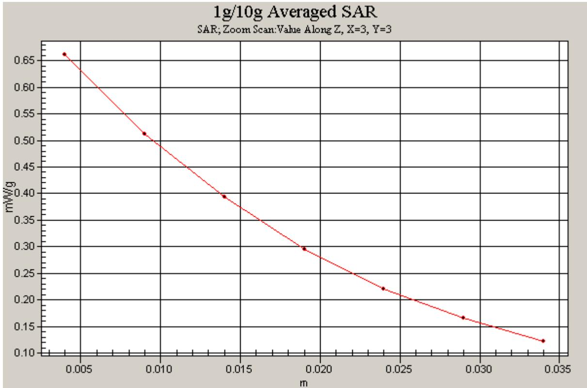
Figure 16 Z-Scan at power reference point (Left Hand Touch Cheek CDMA Cellular Channel 1013)
