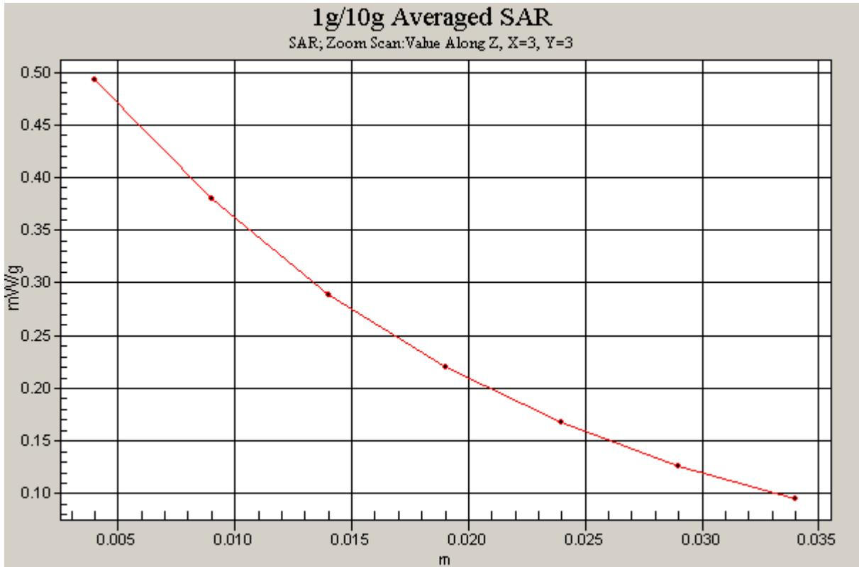
Figure 30 Z-Scan at power reference point (Body, Towards Phantom, CDMA Cellular Channel 384)
