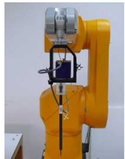
Figure 3 ES3DV3 E-field probe
