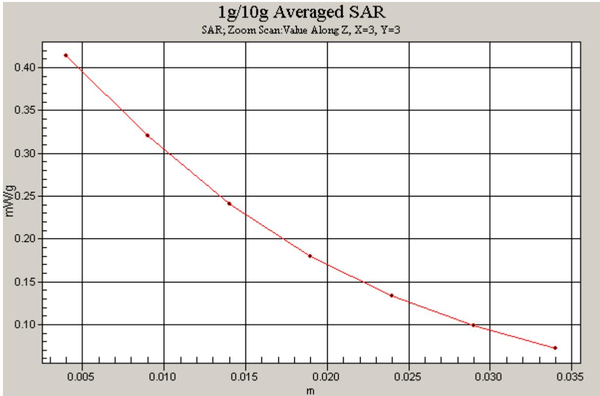
Figure 18 Z-Scan at power reference point (Left Hand Tilt 15° CDMA Cellular Channel 384)
