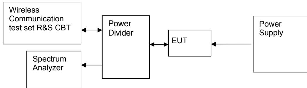
Figure 3. Test Set-up
