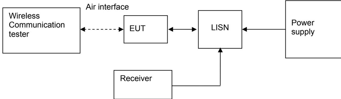
Figure 9. Test Set-up
