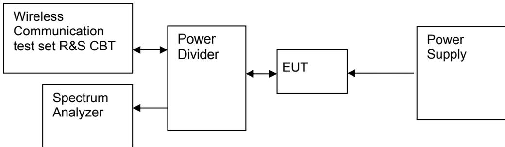
Figure 2. Test Set-up
