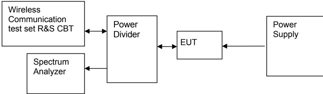
Figure 7. Test Set-up
