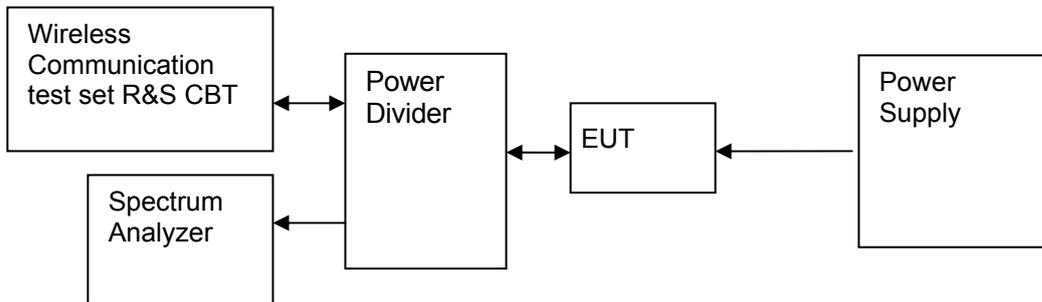
Figure 4. Test Set-up
