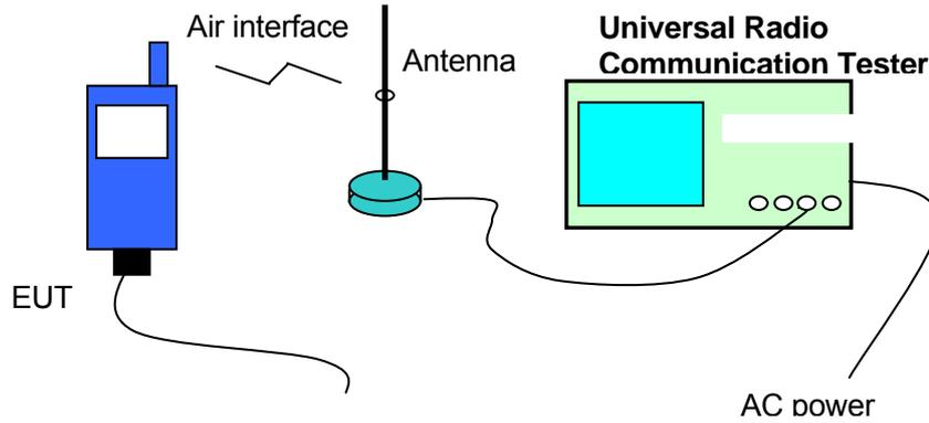
Figure 1.: Test Configuration
