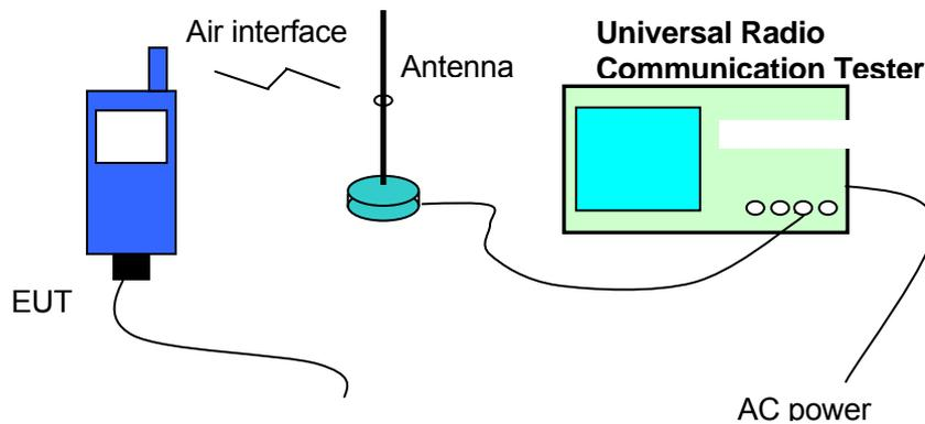
Figure 2. Test Configuration
