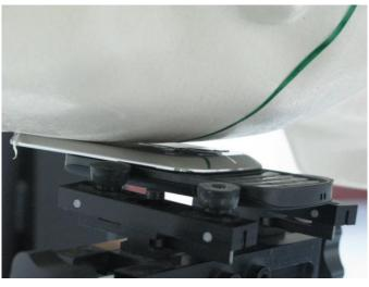
Photo 14: HUAWEI M580 right hand tilted 15° open
