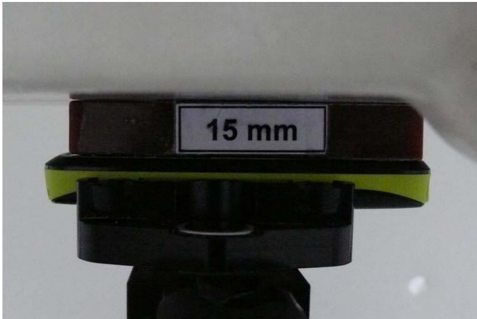
Picture 10: Body, The EUT display towards phantom, the distance from handset to the bottom of the Phantom is 15mm
