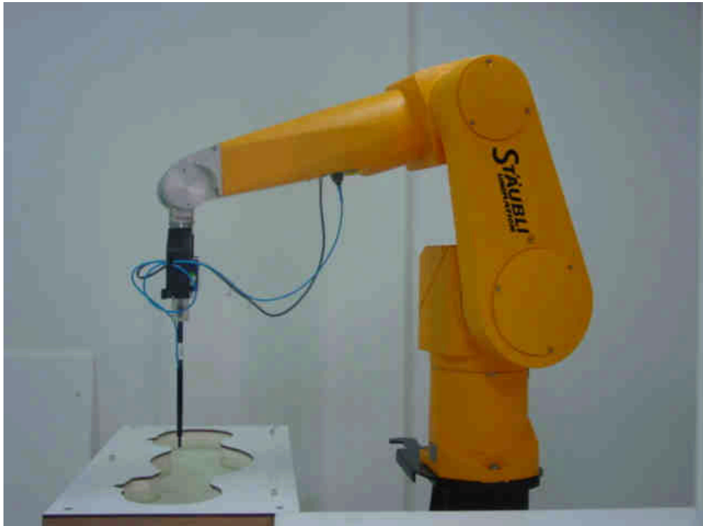
Picture B1: Specific Absorption Rate Test Layout
