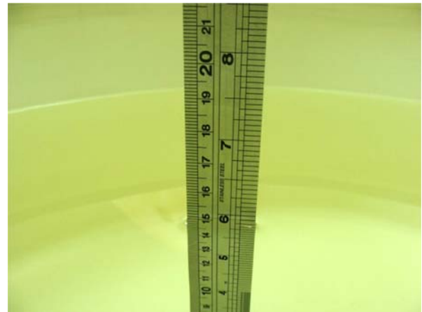
Fig 6.2 Photo of Liquid Height for Body SAR
