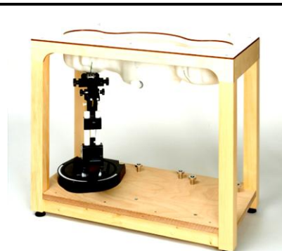
Fig 5.7 Photo of SAM Phantom
