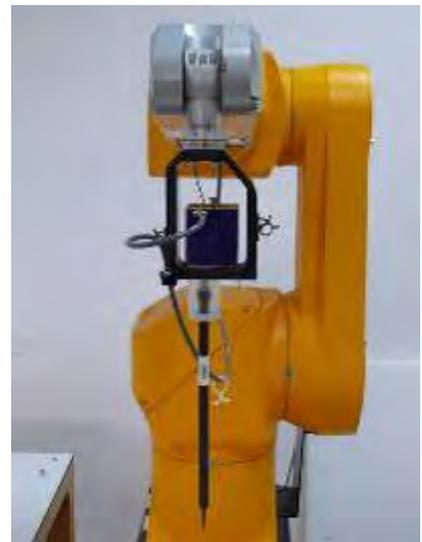
Figure 3. EX3DV4 E-field probe
