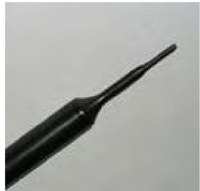
Figure 2. EX3DV4 E-field Probe
