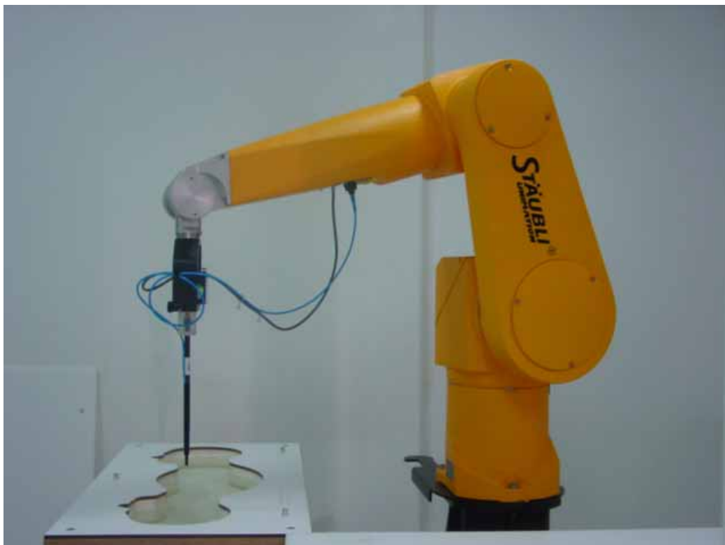
Picture 1: Specific Absorption Rate Test Layout
