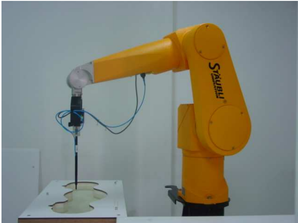
Picture B1: Specific Absorption Rate Test Layout
