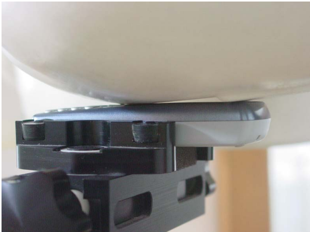
Picture B3: Left Hand Touch Cheek Position
