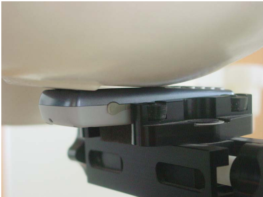
Picture B5: Right Hand Touch Cheek Position
