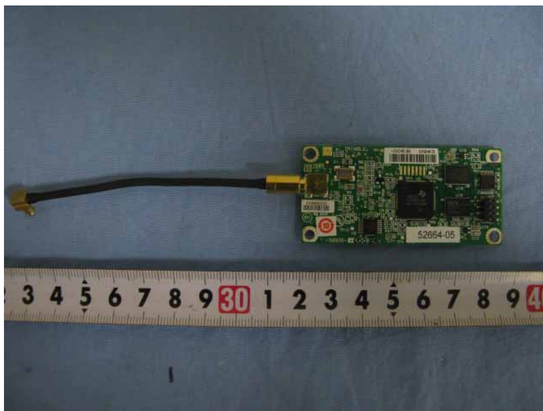
06 View of RF interface board components side
