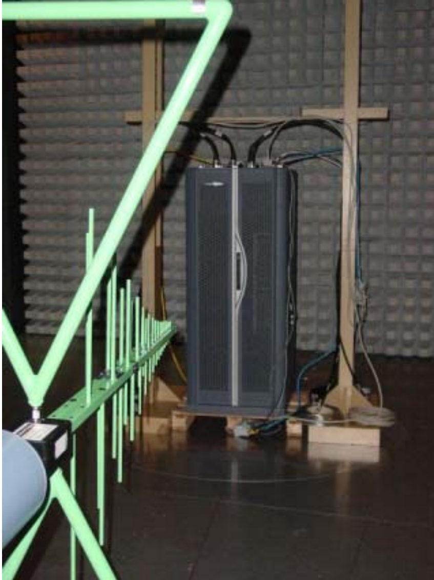
Photo ERP Measurement 30 MHz – 1 GHz
