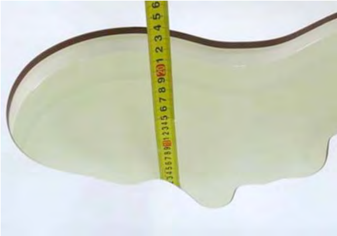
Picture 19: Liquid depth in the head Phantom (5750 MHz, 15.1cm depth)
