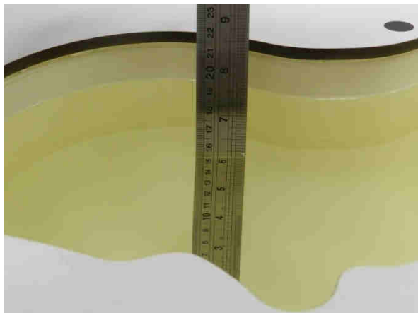
Fig 10.1 Photo of Liquid Height for Head SAR
