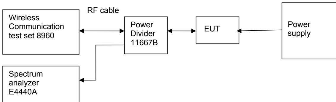
Figure 6. Test Set-up
