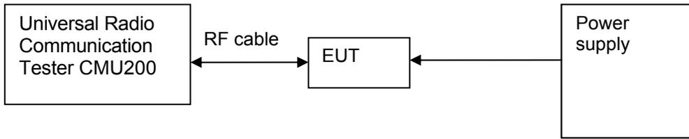
Figure 3. Test Set-up
