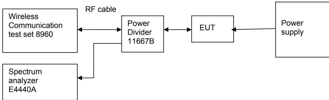
Figure 5. Test Set-up
