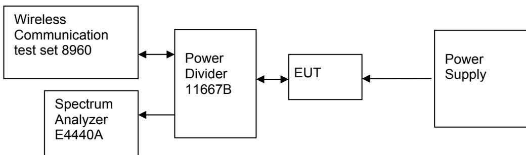
Figure 4. Test Set-up
