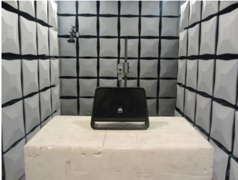
Radiated Spurious Emission (18GHz to26.5GHz)
